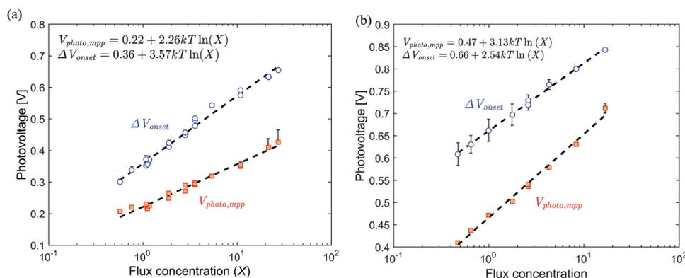
**Figure 5.** The photovoltage at the maximum power point (orange squares) and the photo-induced shift in the onset potential (blue circles) as a function of the flux concentration for a) sample A and b) sample B.
