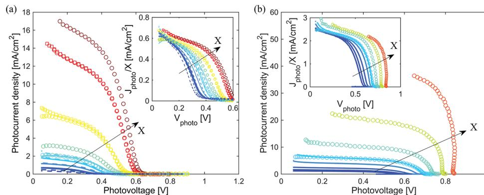
**Figure 3.** The photocurrent density as a function of the calculated photovoltage for various flux concentrations obtained for a) sample A and b) sample B. The insets show the photocurrent density normalized by the flux concentration,  $X$ , as a function of the calculated photovoltage. The symbol and color codes are the same as in Figure 2.
