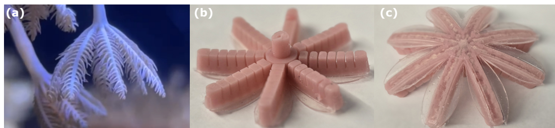
Figure 5.2: (a) Photograph of Xeniidae corals (credit: Anna Dias de Almeida taken at Monterey Bay Aquarium 2024, used with permission) (b) downward and (c) upward view of robot coral.
