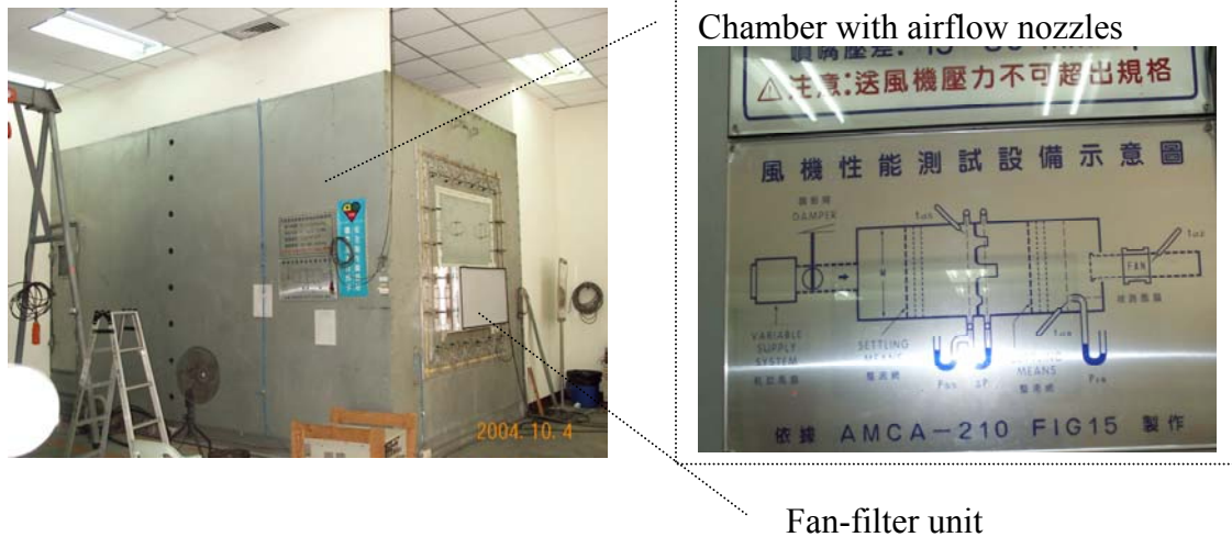
Figure 3 Laboratory measurement layout at the ITRI facility
