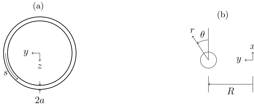
Figure 4.1: (a) Top view of a thin vortex ring and (b) a cross-section view of the xy -plane. The ring moves in the x -direction ( \theta = 0 ).
