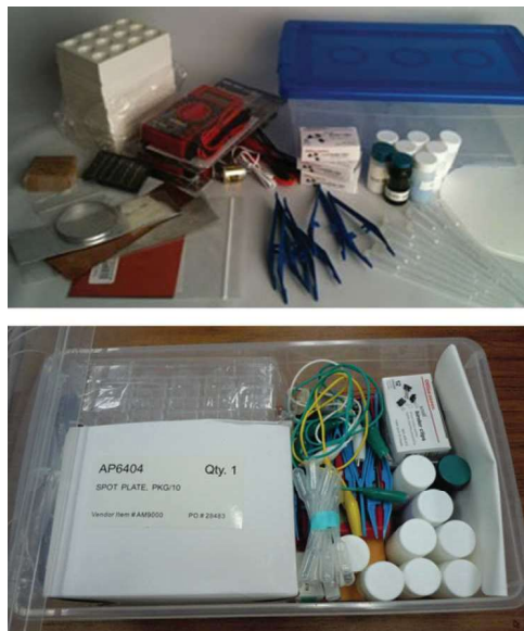
Fig. 8. Images of part of an early version of the assembled JfJ kits, which included multimeters, well plates, pipettes, tweezers, binder clips, and vials of chemical compounds that were used for the chemistry and solar cell modules.
