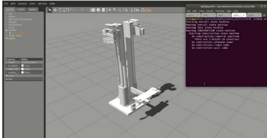
Figure 57: Robot model in the Gazebo environment, running the construction state machine
