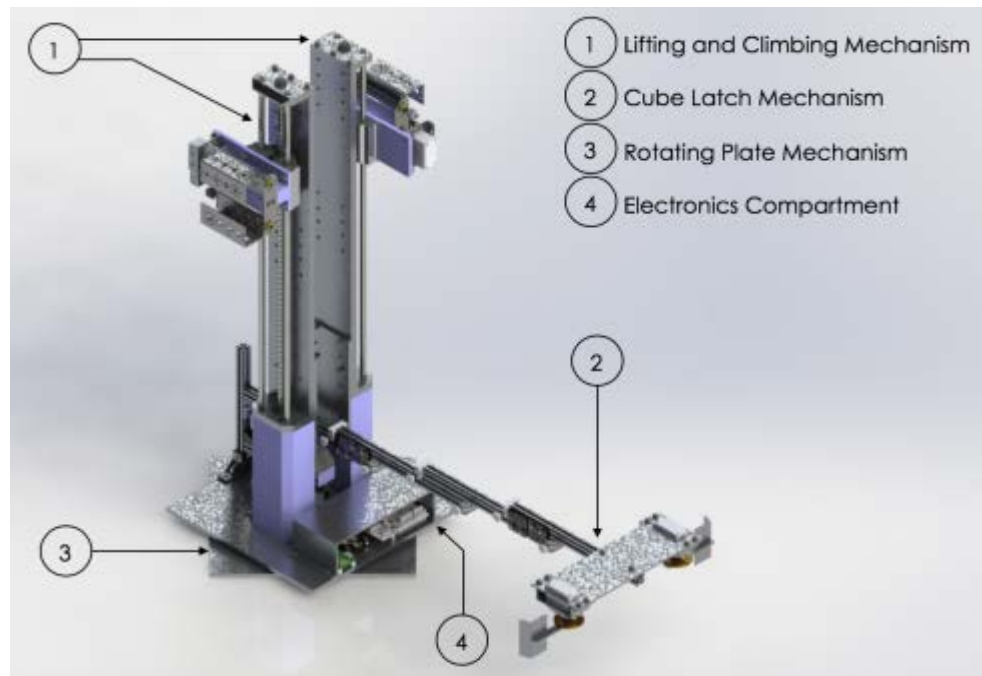
Figure 1: The final robot design featuring its main components.
