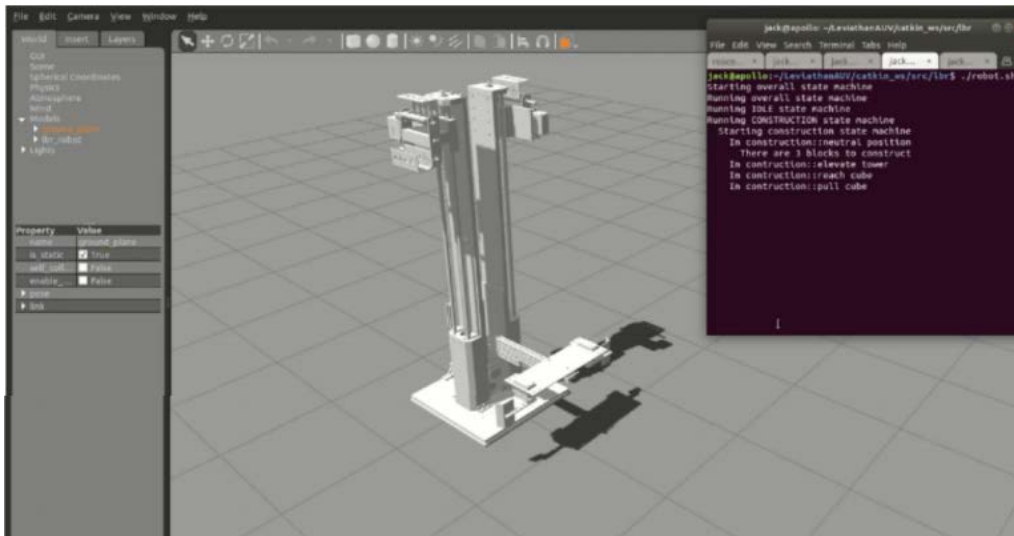
Figure 35: Robot model in the Gazebo simulation environment running the construction state machine.
