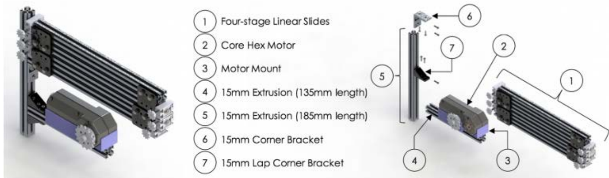
Figure 15: (Left) isometric view and (right) exploded view of the linear slide assembly
