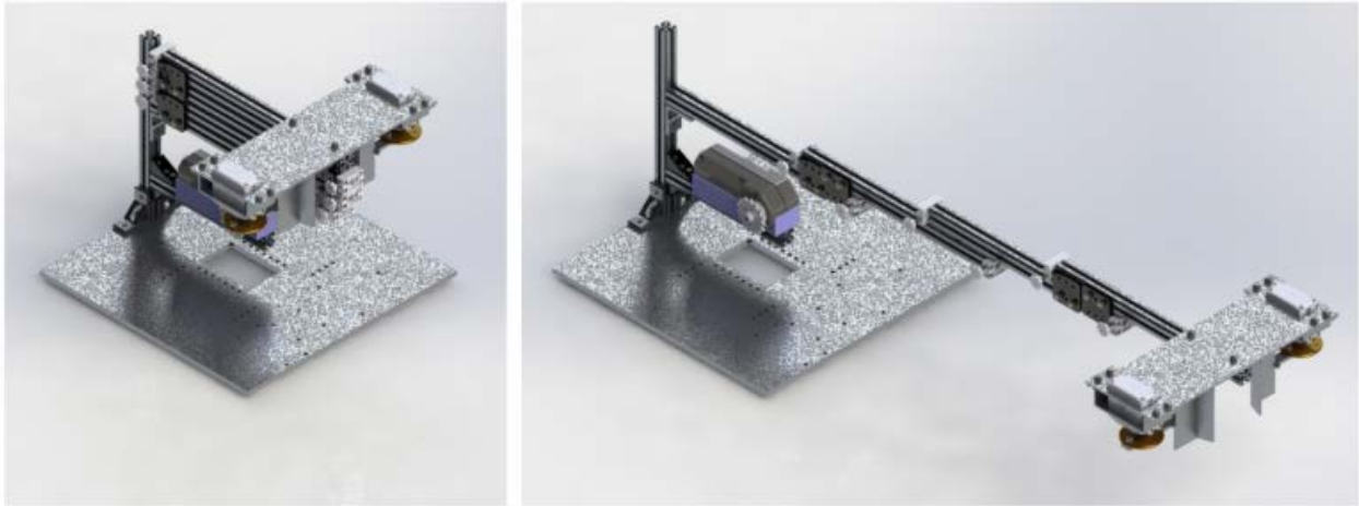
Figure 12: Isometric view of the cube latch mechanism when it is (left) retracted and (right) extended
