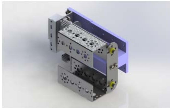
Figure 8: (Left) isometric view and (right) exploded view of the linear actuator
