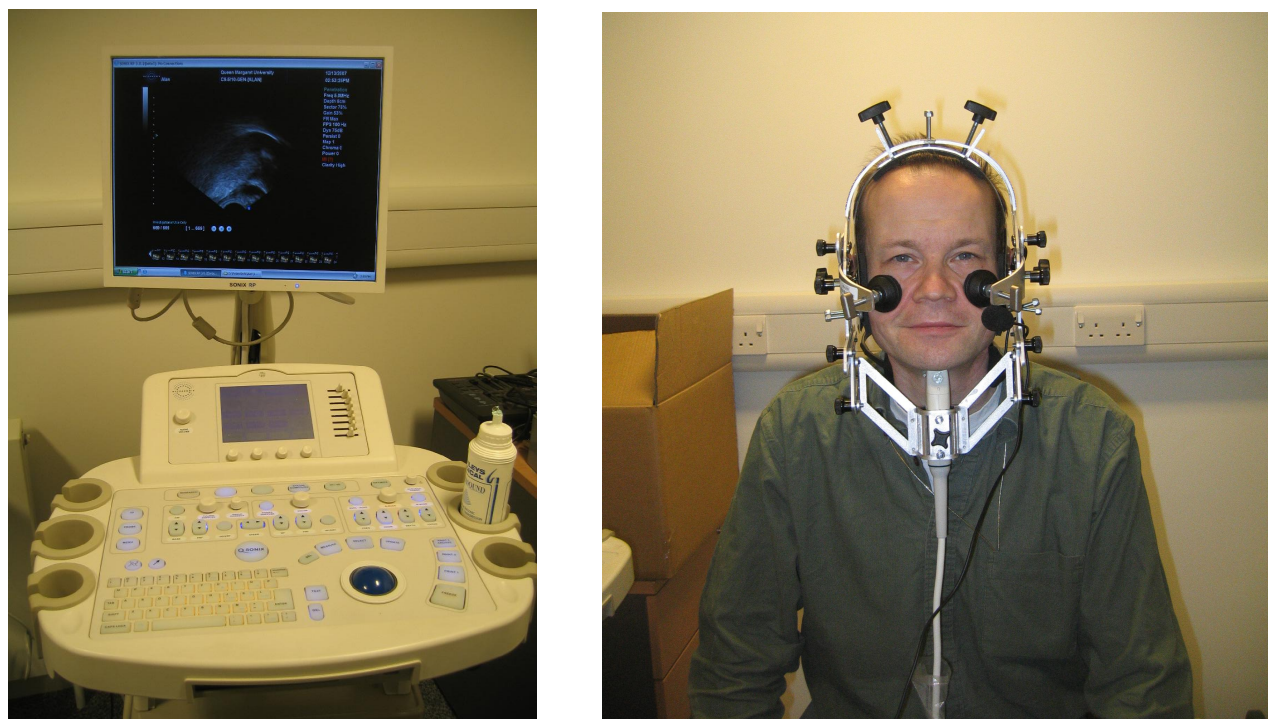
Figure A.4: Left: 2D ultrasound machine used. Right: device to stabilize the head (to reduce motion w.r.t. the ultrasound probe) [133].
