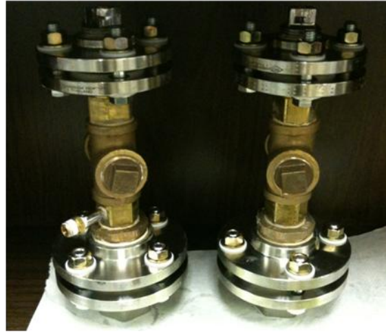
Figure G-4. Photo of the heater head fittings for the CIET Test Bay.
