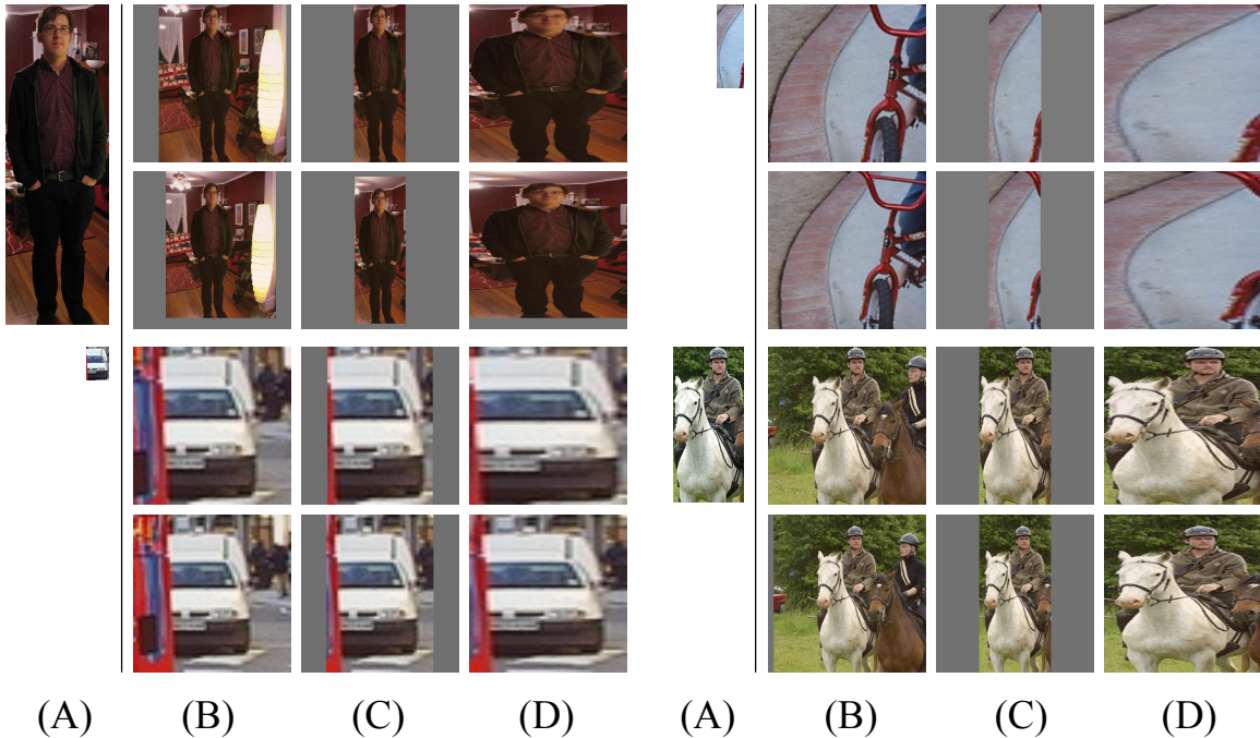
Figure 3.7. Different object proposal transformations. (A) the original object proposal at its actual scale relative to the transformed CNN inputs; (B) tightest square with context; (C) tightest square without context; (D) warp. Within each column and example proposal, the top row corresponds to p = 0 pixels of context padding while the bottom row has p = 16 pixels of context padding.
