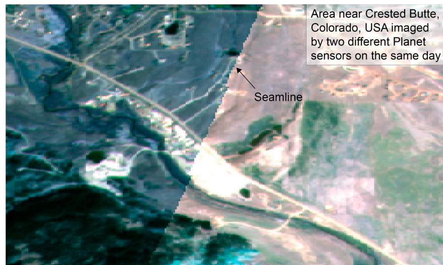
Figure 2. Example of sensor spectral differences in PlanetScope sensors that impact potential replicability of studies.
