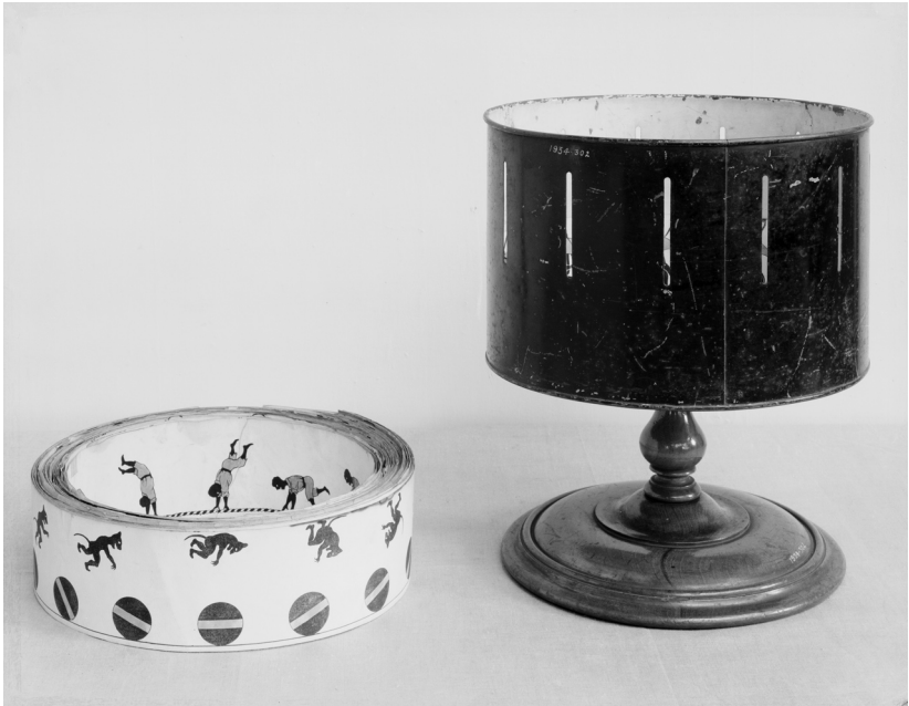
FIGURE 21. Original zoetrope, ca. 1860s. A zoetrope is a cylinder with a series of pictures on the inner surface that, when viewed through slits with the cylinder rotating, give an impression of continuous motion. The idea that a sequence of drawings should be made on a band of paper to be viewed in a rotating cylinder was first suggested by Simon Stampfer in 1833. However, it wasn't until the 1860s, when several patents were obtained, that the zoetrope appeared on the market. It remained a popular parlor toy for the rest of the century. © Science Museum / Science & Society Picture Library—All rights reserved.
