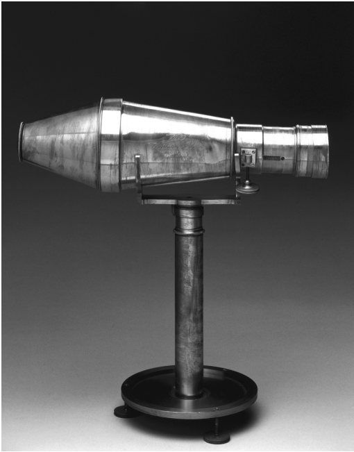
FIGURE 33. Replica of a camera designed by Peter Voigtlander in 1841. It is one of the earliest practical portrait cameras and one of the earliest cameras made of metal. The body consists of two cones, the longer of which forms the camera itself and contains the lens. The smaller cone contains the focusing screen and eyepiece. © National Media Museum / Science & Society Picture Library—All rights reserved.
