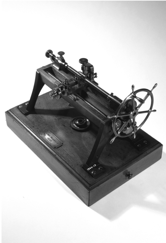
FIGURE 28. Model of the original screw-cutting lathe by Henry Maudslay. This model is arranged to be driven by hand power. The workpiece on which the screw is to be cut is carried between head- and tailstock, with the lead screw mounted in the lathe bed. The slide carries the tool holder, connected to the lead screw. The depth of the cut is controlled by a hand wheel, and a set of change wheels allows for a range of different threads. © Science Museum / Science & Society Picture Library—All rights reserved.
