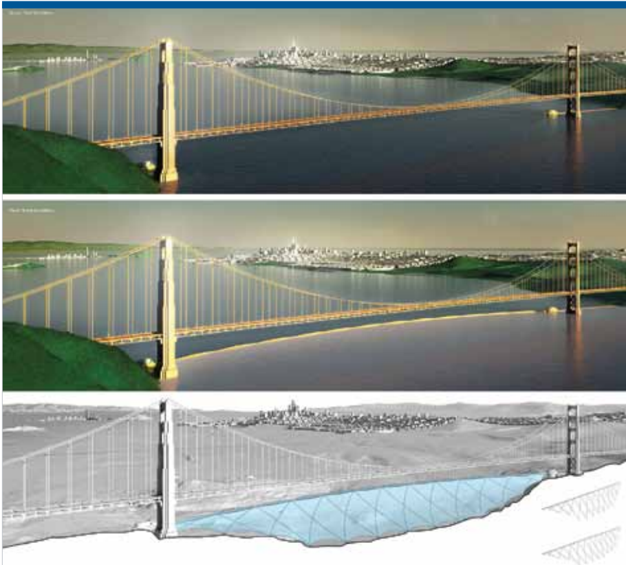
Figure 5.4 Proposed Barrier to Control Sea Level Rise Inside the Golden Gate, BCDC Rising Tides Competitor Winner
