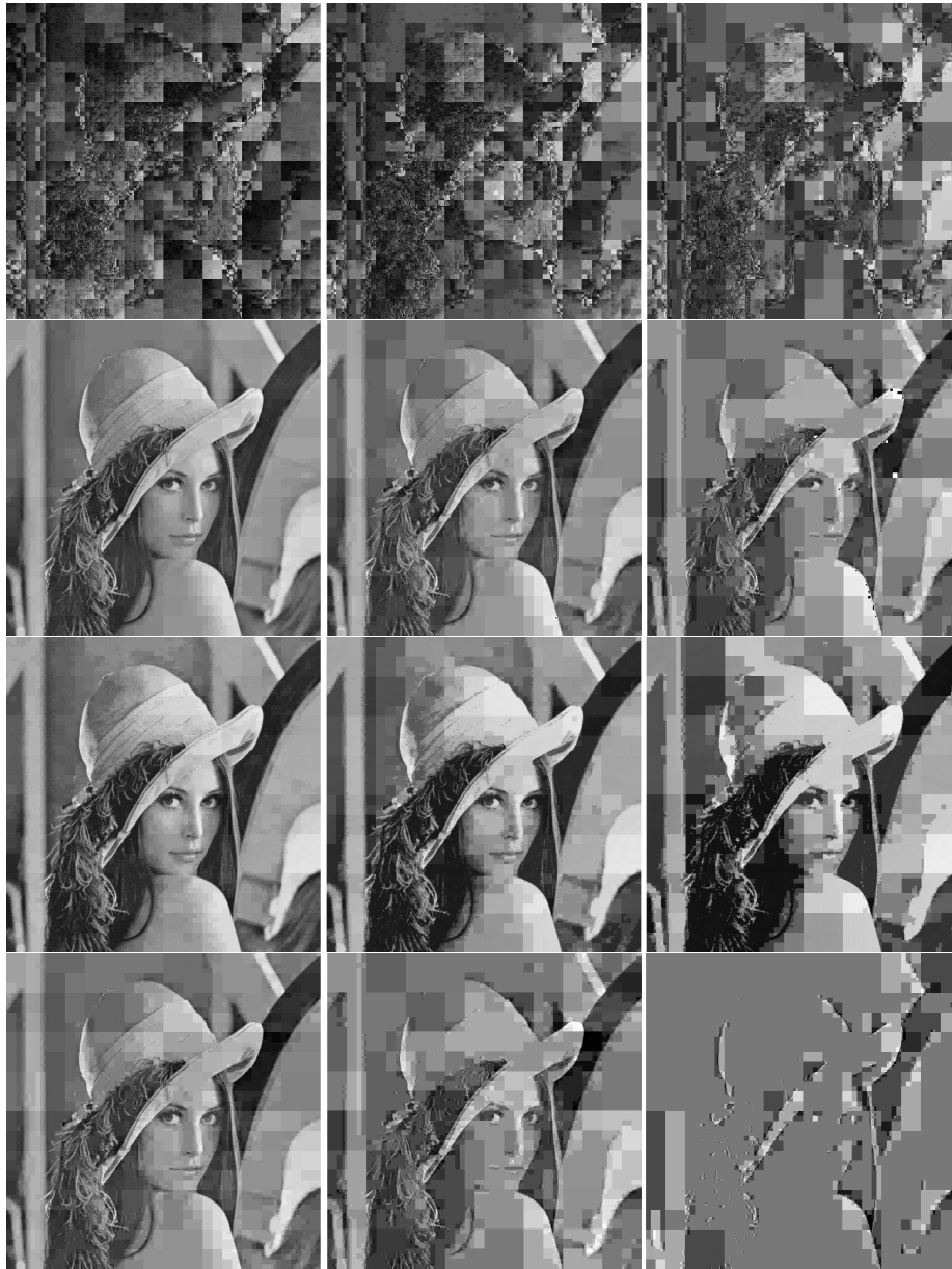
Figure 15. “Lena”, quantized to 5, 4, and 3 bits. From the top: TLHaar, CFH, PLHaar, and S–Transform.
