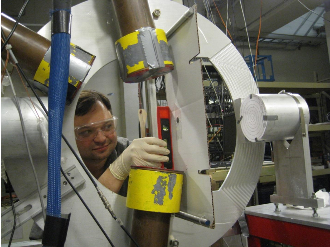
Figure 3.12. Detector holding rig installation. Detectors are rigidly mounted at \theta = 100 and \theta = 150 . The whole assembly rotates between \varphi = 0 and \varphi = 90 .
