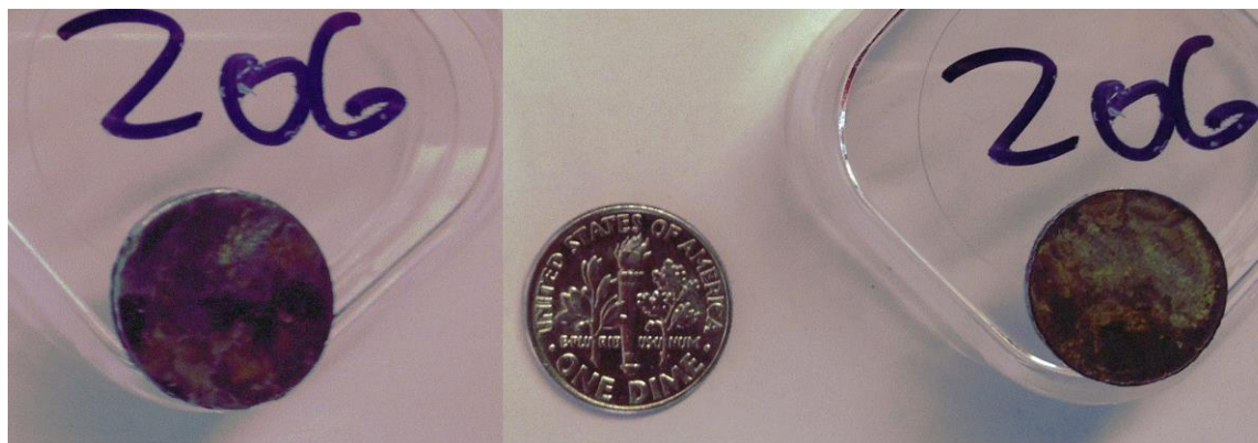
Figure 3.4. The Lead 206 target from both sides, next to a dime for a scale comparison.
