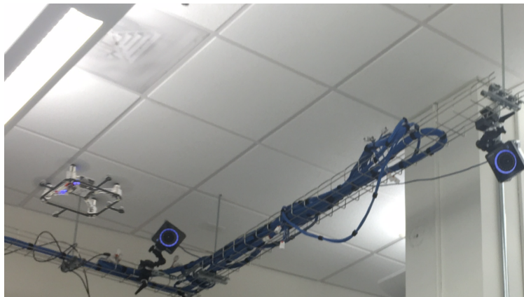
Figure 7.8: A Crazyflie 2.0 flying during our hardware demonstration. Two OptiTrack cameras are visible in the background.
