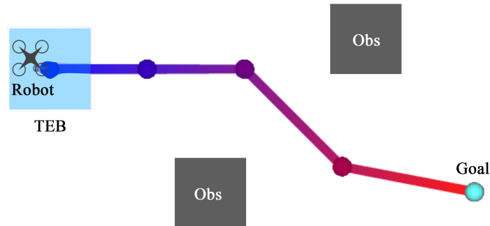
Figure 9.4: Top-down view of FaSTrack applied to a 6D quadcopter navigating a static environment. Note the simple planned trajectory (changing color over time) and the tracking error bound (TEB) around the quadcopter. This TEB is a 6D set that has been projected down to the position dimensions. Because we assume the quadcopter moves independently in (x, y, z) , this projection looks like a box, making collision-checking very straightforward.
