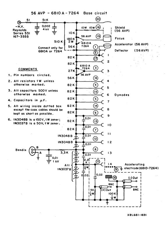
Fig. 3. Base circuit diagram.
