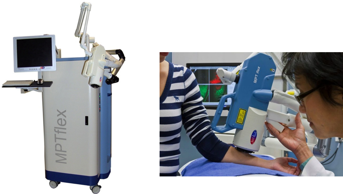
Figure 1. MPTflex - laser-scanning multiphoton microscopy - based clinical tomograph
