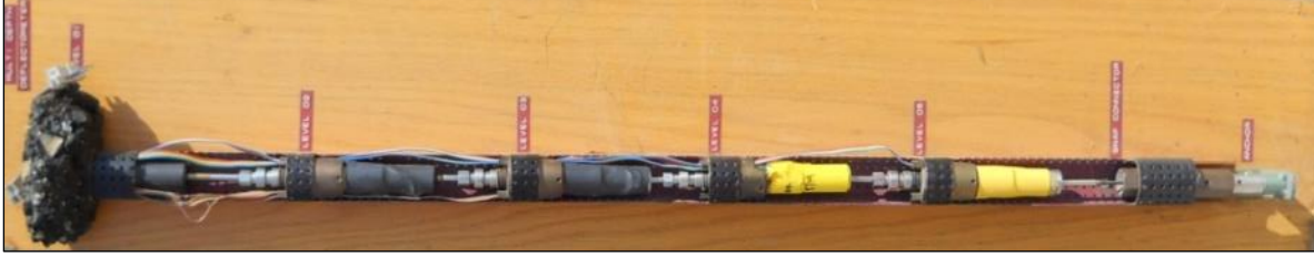
Figure 4.5: A model multi-depth deflectometer (MDD), showing five modules.
