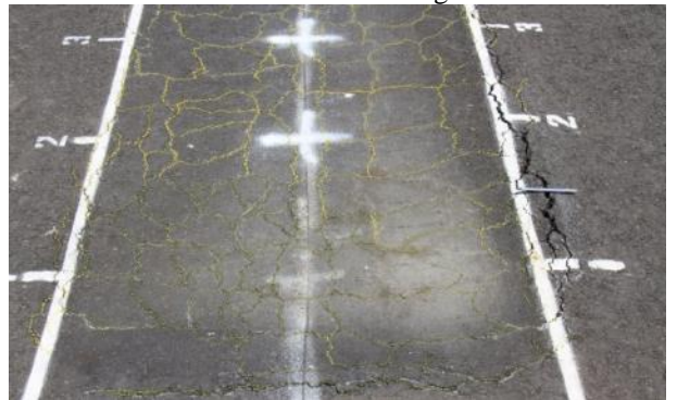
Cracking and deformation at end of test section
