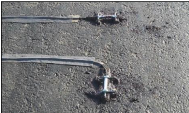
Figure 4.3: Strain gauge installation.
