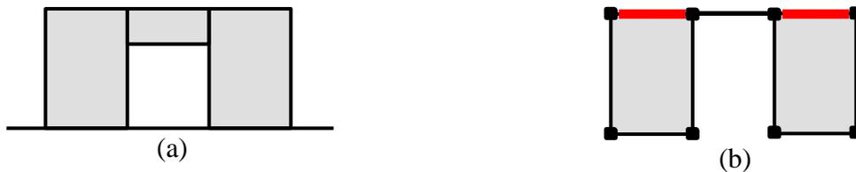
Figure 4-12. (a) Schematic drawing of a coupled wall system, (b) Perform 3D modeling of shear walls, coupling beams and embedded beams
