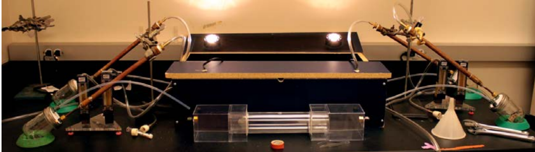
Figure 2.1: The final olfactometer design. A two-choice olfactometer comprised of an acrylic tube with funnels leading to terminal collection boxes. These were connected with Teflon tubing to a jar containing the odor source or control. Air was pulled through the system by a vacuum source connected to an outlet in the top of the central chamber.
