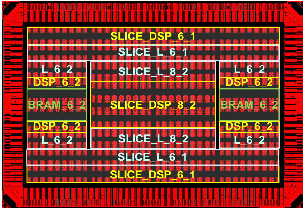
Figure 5.9: Top-level layout floorplan of the 2048-LUT FPGA with 512 CLBs.
