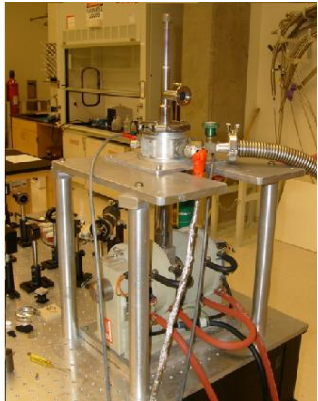
Fig. 5-8 Continuous Flow Cryostat Chamber. Schematic of the system (left). Picture of the system with pump and electro-magnet (right).
