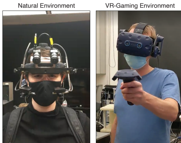
Figure 3.1: Apparatus for the natural and VR-gaming environments. Left: Apparatus for measuring disparities and eye movements in the natural environment. The custom head-mounted device has two cameras and a binocular eye tracker. A backpack contains the host computer and power supply. Right: HMD used to measure eye movements and disparities in the VR-gaming environment. Handheld controller enables game interaction.
