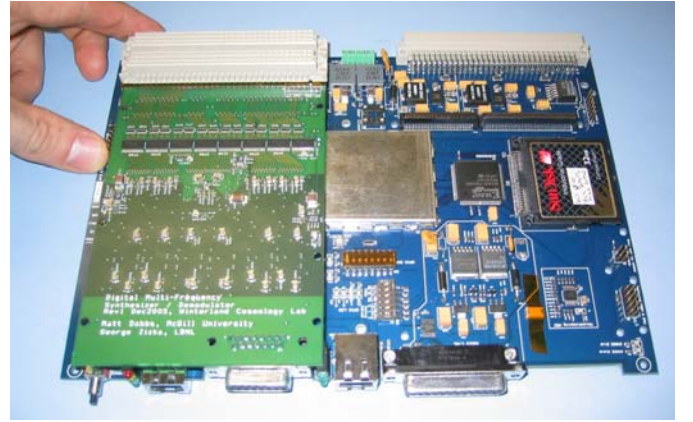
Figure 2 An FPGA motherboard is shown with one of its two analog converter mezzanine boards attached.
