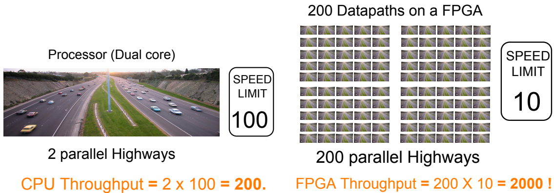
Figure 1.1: Demonstration of the throughput of a CPU and FPGA: A Highway Analogy. An FPGA with a ten times slower clock rate can offer 10X the throughput of a dual core CPU by implementing two hundred parallel data paths on the fabric.
