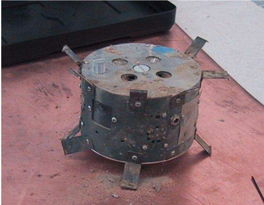
Figure 9.11: An SHM node built by the SAIC-led SHM team, including Sensoria, Ensign-Bickford, and Universal Propulsion. The node is 12cm in diameter. The top and bottom each have four solid-propellant rocket thrusters capable of moving the node approximately 8 meters in one of the four cardinal directions. The four holes on the top of the unit are the thruster nozzles. Photo courtesy of Sensoria Corporation.
