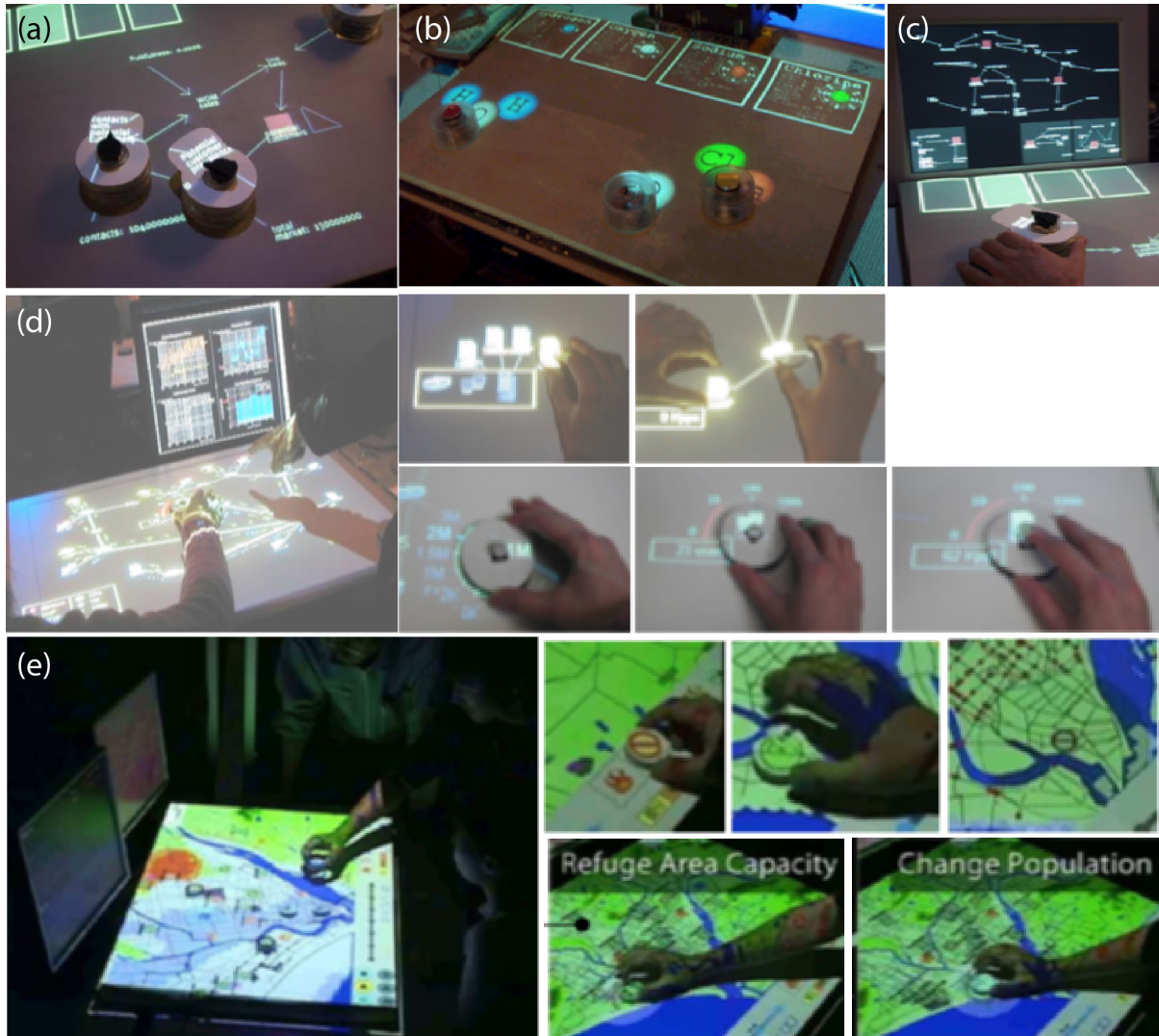
Figure 2.19: The applications of tangible user interfaces (TUIs) for computer simulations are as follows: (a) Sensetable can be applied for (b) chemical reaction simulation and (c) system dynamics simulation, as demonstrated by Patten [59]. (d) In a network simulation, tangible interactions allow for the modification of client and server settings [69]. (e) In a disaster simulation system, parameters such as refuge area capacity or population can be adjusted by grabbing and turning pucks, as illustrated by Kobayashi et al. [70]. Both (d) and (e) are presented by Kobayashi et al. Images reproduced with permission.
