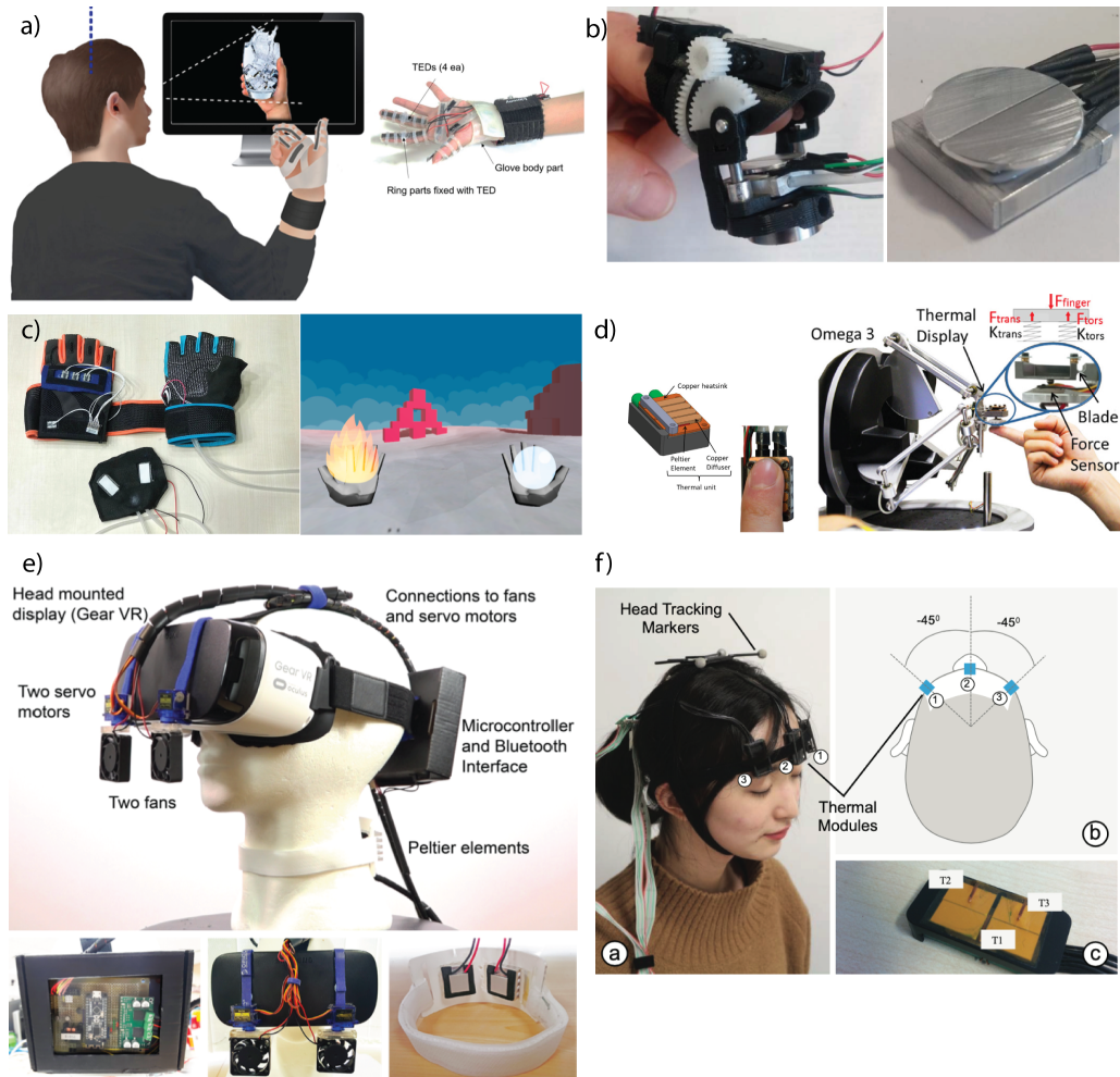
Figure 2.16: Thermal devices are widely used in VR applications. (a) Kim et al. developed a flexible thermal glove for VR interaction. This glove enables users to engage in haptic interactions such as grasping and pinching virtual objects, utilizing thermal feedback [48]. (b) The thermal module is integrated into the Haptic Thimble, an existing haptic device. This device provides heat sensations to the fingers, rendering thermal feedback in VR experiences [49]. ©2018 IEEE. (c) Chernyshov et al. developed thermal feedback displays on the hand within virtual environments to reduce the time delay of thermal feedback [50]. (d) Gallo et al. developed a small thermal display that can be integrated into existing haptic devices like Falcon and OMEGA3. This compact thermal display leverages the capabilities of other haptic devices to provide multiple sensory properties [51]. ©2015 Gallo, Rognini, Santos-Carreras, Vouga, Blanke and Bleuler. (e) Ambiotherm is a thermal device used in conjunction with a VR head-mounted display (HMD). The thermal module is attached to the neck, allowing the ambient temperature in the virtual environment to be rendered through thermal feedback [52]. (f) Peiris et al. used thermal feedback on the forehead to enhance spatial awareness in VR experiences [53]. ©2017 IEEE. (a) is licensed under Creative Commons 4.0. Images reproduced with permission.
