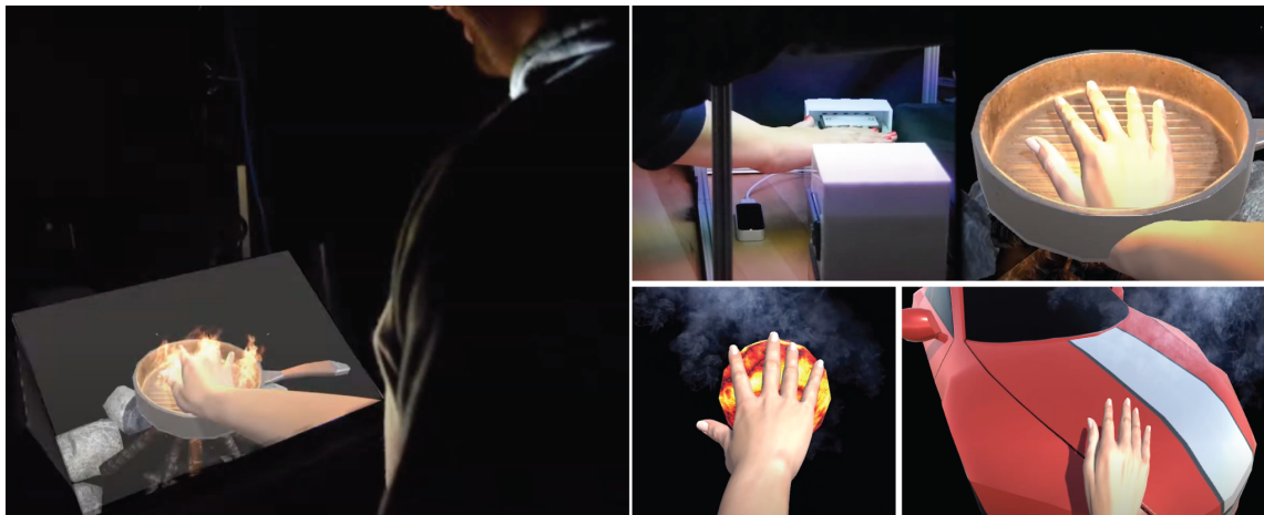
Figure 6.13: Impossible Touch represents a compelling use case of the Thermal Grill illusion within the realm of virtual reality, specifically in augmented haptic reality. By thermal feedback to create a sensation of fake burning heat, users are able to interact with objects that would typically be too hot to physically touch with their hands in Virtual Reality and experience fake burning heat.
