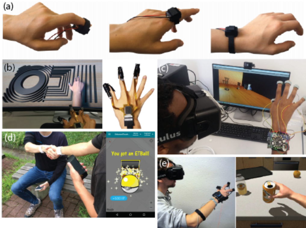
Figure 2.15: The wearable display can be attached to various body parts, including the finger, hand, wrist, and other body parts. (a) The Haptic Ring provides vibrotactile feedback for rendering textures. The ring can be attached to the tip of the finger, finger phalanx, and wrist as well [45]. ©2019 IEEE. (b) FinGAR is a finger glove designed for augmented reality. It utilizes a DC motor attached to the finger to provide sensations of macro roughness, friction, fine roughness, and hardness [36]. ©2017 IEEE. (c) The finger-worn device aims to modify stiffness using vibrotactile feedback during interactions with virtual objects [46]. ©2017 Maereg, Nagar, Reid and Secco. (d) EnhaunchedTouchX is a smart bracelet designed to augment interpersonal touch interactions. During hand-to-hand touch interactions, vibrotactile feedback is transferred from one hand to the other [43]. (e) HapTip enables multi-finger interaction in VR environments and provides sensations of a rough virtual surface, inertia, or weight of virtual objects [47]. ©2016 Girard, Marchal, Gosselin, Chabrier, Louveau and Lécuyer. Images reproduced with permission.
