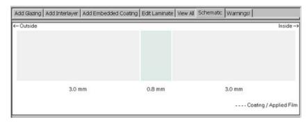
Each layer is drawn in correct relative scale, and is drawn in the color of light transmitted through that layer (if color averages are available in the selected standard). The thickness of each layer is shown, unless the text will not fit, in which case the thickness text will not display. The gap width for glazing systems is shown to scale, and can be set (see "Gap Width in Glazing Systems" on page 40).
