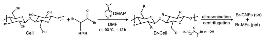
Scheme 1 2-Bromopropionyl esterification of cellulose and ultrasonication of Br-Cell to generate hydrophobic Br-CNFs in the supernatant and Br-Cell microfibrils in the precipitate.
