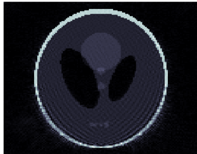
(c) Phantom reconstruction without field map correction
