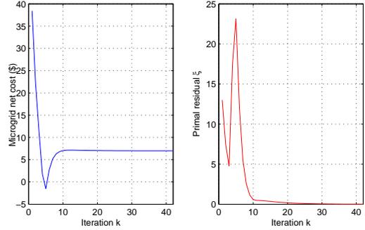
Fig. 3. Convergence of the net cost and evolution of the primal residual.
