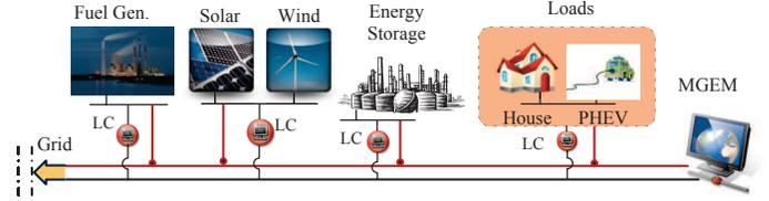
Fig. 1. Decentralized infrastructure of a microgrid with communications (black) and energy flow (red) networks.
