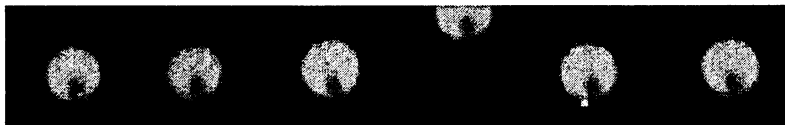
Fig. 3: A series of snapshots of a 2 \mu\text{m} latex sphere tracked by active feedback
