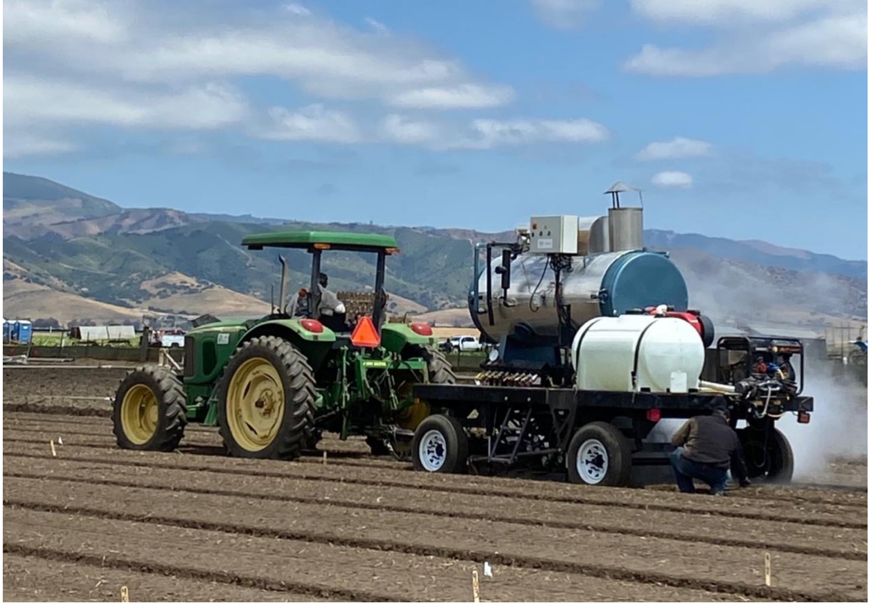
Figure 2.1 Band steam applicator used in trials 1 to 5.
