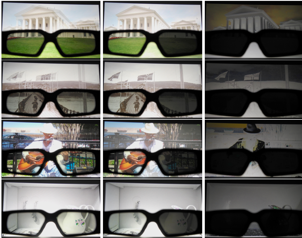
Figure 2.11: Here we show several examples of our prototype in use. In each image, the projector screen is visible directly at the top of the image, and through each lens of the stereo glasses at the bottom of the image. (Left Column) A typical 3D display (Middle Column) our 3D+2D prototype, with \alpha_R = 30\% (Right Column) the 3rd channel we display to cancel out the right-eye image. Images used with permission from Flickr users GammaMan, Trondheim_Byarkiv, and Isaiah-v.
