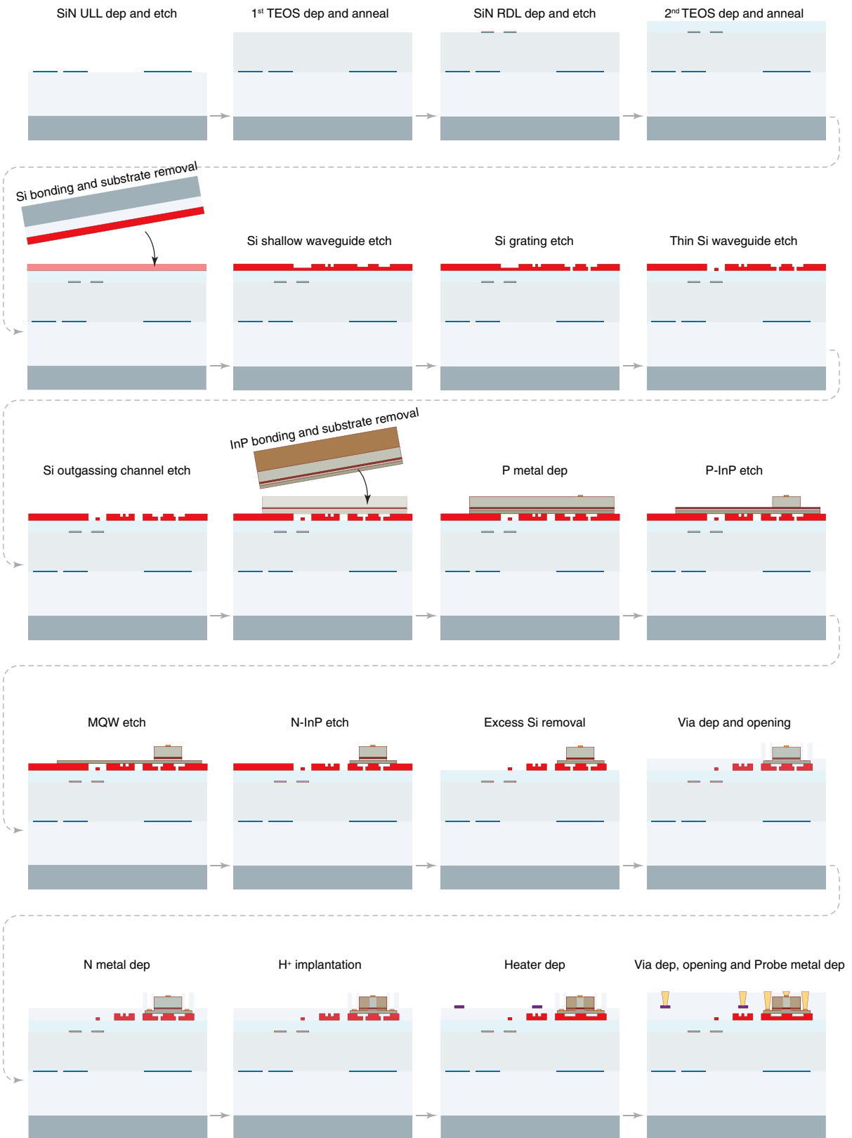
Extended Data Fig. 7 | Detailed process flow charts. The details of the respective layers can be found in Fig. 1. The difference in the III-V/Si section between the last two charts and the previous charts are illustrations of the etched Si grating.
