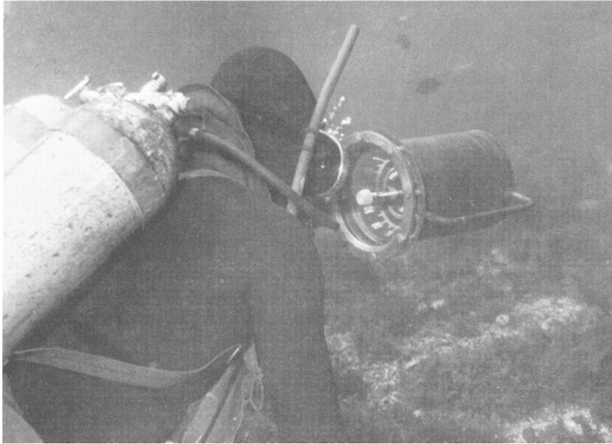
FIGURE 2 Biologist-diver Charles H. Turner horizontally surveying the sea floor with a diver-held fathometer. Photo by Earl E. Ebert.
