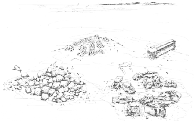
FIGURE 1 Artists concept of a multi-component study reef placed in Santa Monica Bay; 60-foot depth.
