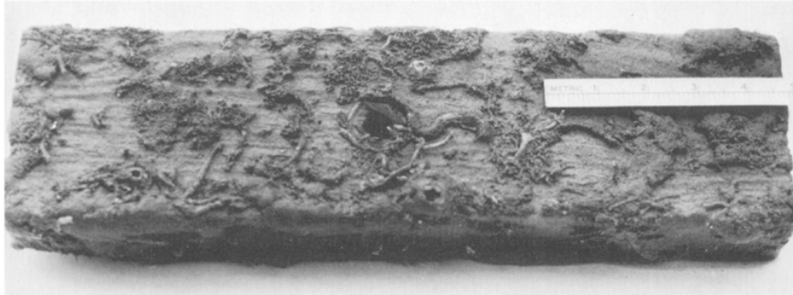
FIGURE 32 One of the test blocks placed on the WCB reefs. Note the serpulid worm tubes and the beginning mat-like layer of Victorella argilla (ectoproct). Photo by Robert R. Given.
