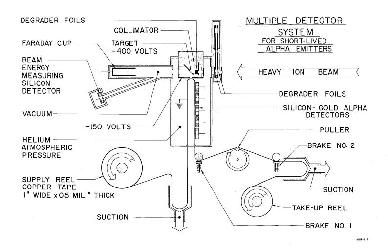
Fig. 1. Schematic diagram of apparatus.
