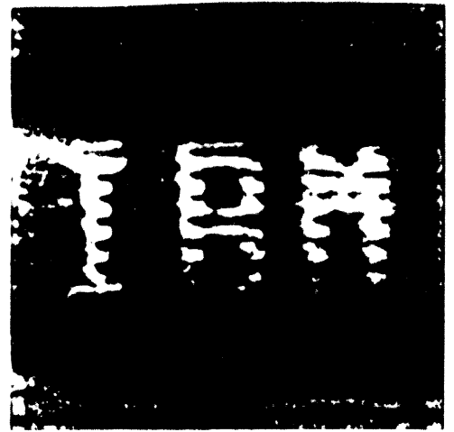
Figure 2 (a) AFM image of a pit written in PMMA. Pit is roughly 300 nm in diameter (b) AFM image of the IBM logo written between the grooves of an optical disk. The individual pits are approximately 100 nm in diameter.
