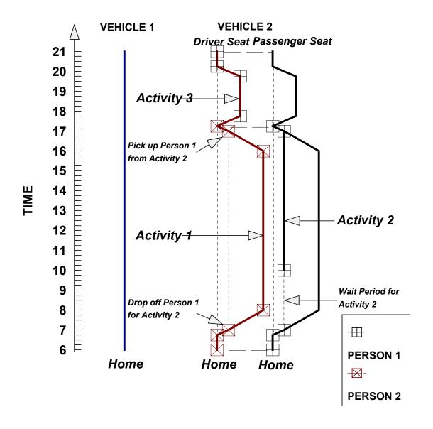
**Figure 6.** Optimal Time-Space Path, Vehicle, Activity Allocation, and Model Choice for CASE 5 Example
