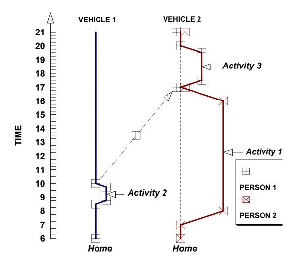
**Figure 5.** Optimal Time-Space Path and Vehicle and Activity Allocation for CASE 4B Example
