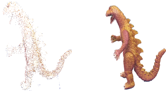
Fig. 1. An initial sparse reconstruction, with good camera estimation, on the left. It can be made into a very dense version, on the right, by our method.
