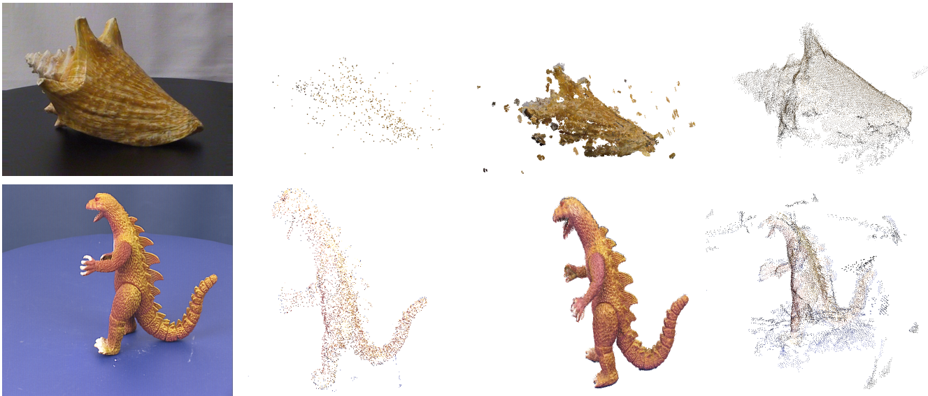
Fig. 5. Results from the proposed method for the Dinosaur and Conch datasets. The first column shows an example input image, the second shows the initial sparse reconstruction used as input, the third shows results from the proposed method, and the last column shows the result of CMVS/PMVS as implemented by VisualSfM. For the Conch shell dataset with 216 images of size 640x480, our method takes 3 minutes. For the Dinosaur dataset with 36 images of size 720x576, our method takes 1.3 minutes.
