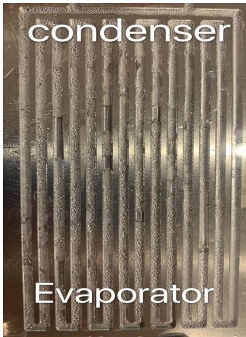
Figure 15. Demonstration of working fluid oscillating in the pipe
