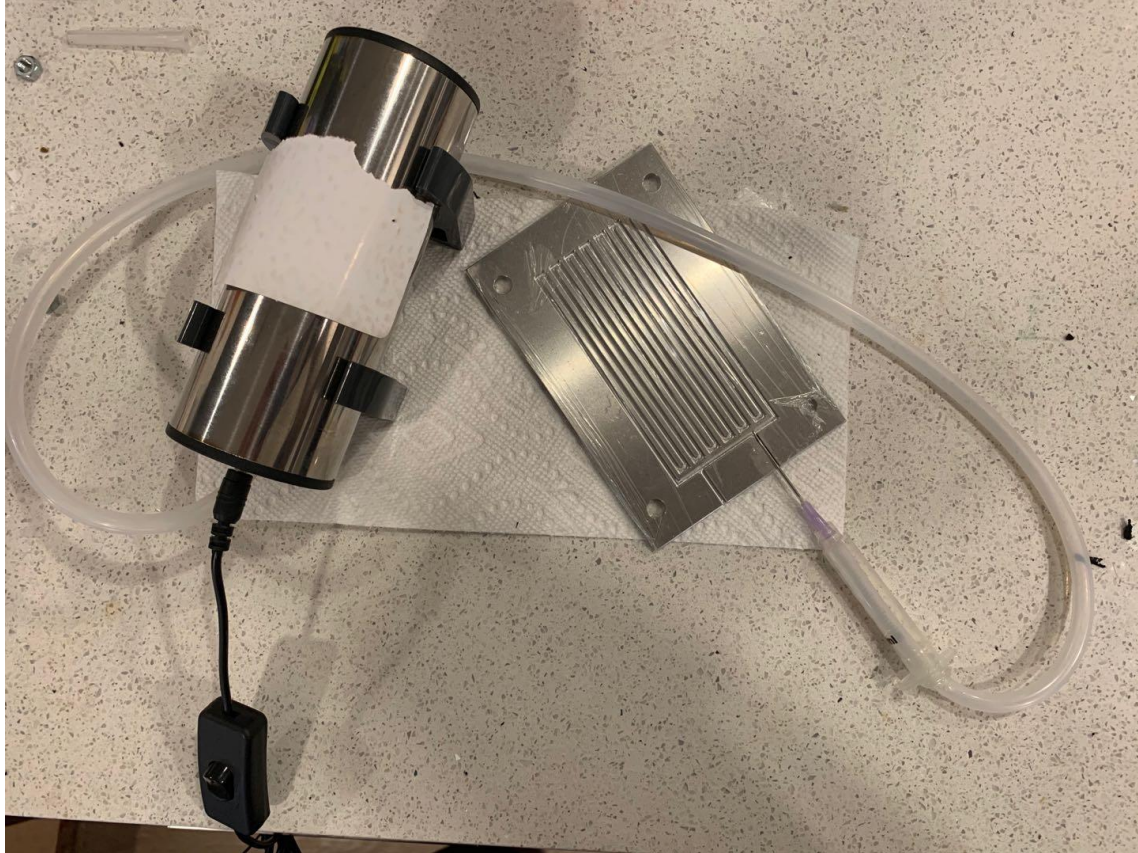
Figure 13. Vacuum Pump connects with the OHP
