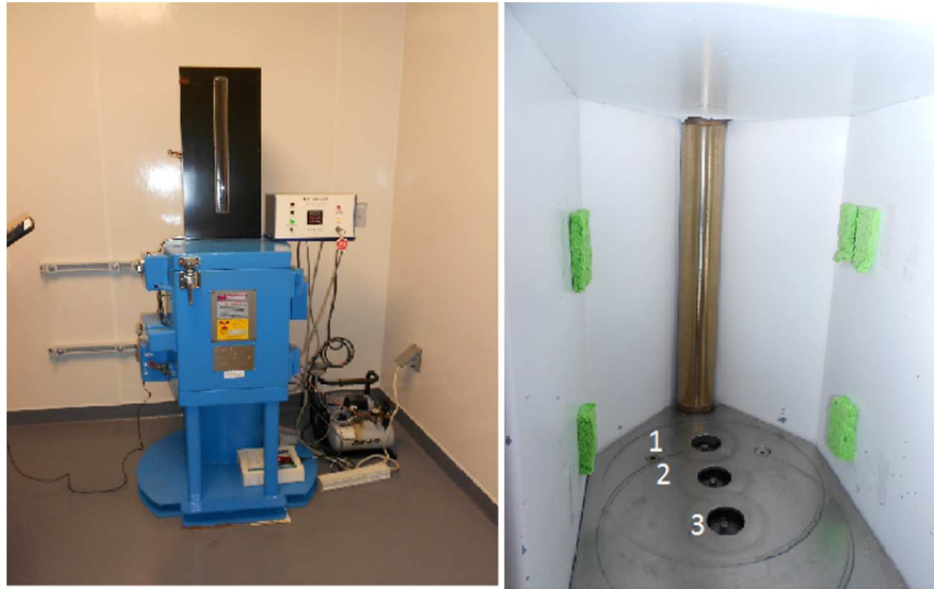
Figure 2. 1. J.L. Shepherd and Associates Mark I-68A 4000Ci Cs-137 irradiator and each irradiator drive shaft position.
