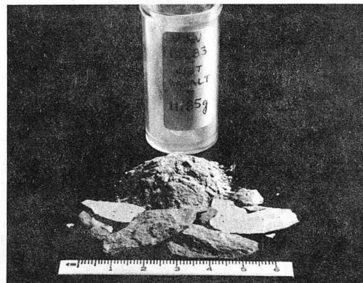
Fig. 7 - a) Napa basalt bombarded by single 4 MV electron pulse. b) The spall debris therefrom.
