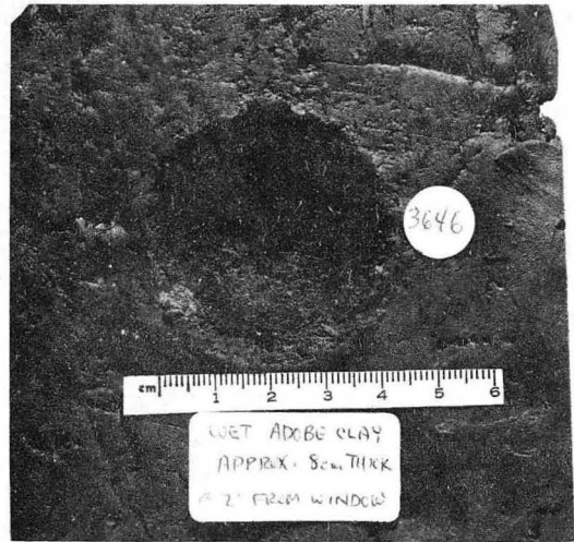
Fig. 6 - Moist adobe clay subjected to single 2 MV electron pulse.
