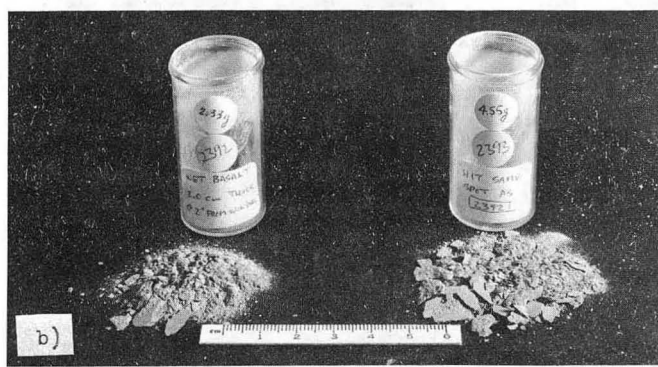
Fig. 3 - a) Napa basalt bombarded by two 1.1 MV electron pulses on same spot. b) The spall debris therefrom.
