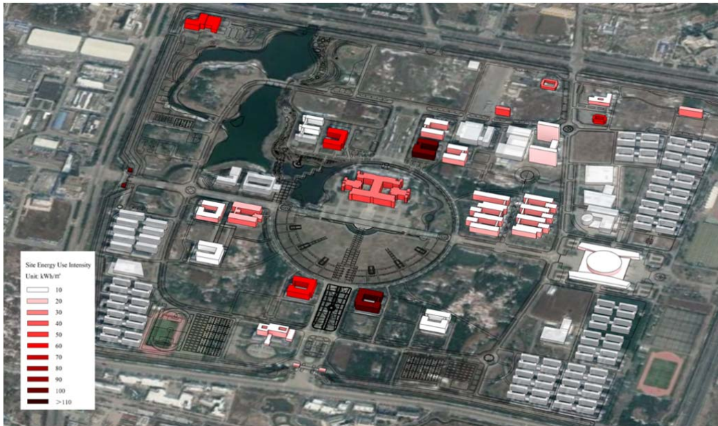
Fig. 5. The average building EUI results distribution on the SEU new campus.
