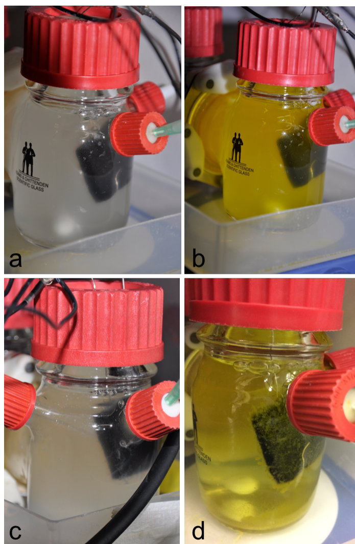
Figure 4.12: Photographs of bioreactors at time of DSSN+ addition ( t = 3.6 h) and at t = 12 h. At t = 3.6 h, bioreactor solutions were visibly turbid at OD_{600nm} = 0.55 \pm 0.04 for all (a) untreated and (b) DSSN+ treated bioreactors. After overnight operation ( t = 12 h) solutions from (c) untreated bioreactors were still visibly turbid, while solutions from (d) DSSN+ modified bioreactors were visibly less turbid with cell mass adhered to electrodes.
