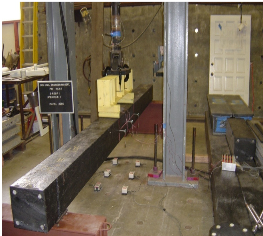
Figure (3.4): Typical four-point bending test setup
