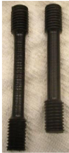
Figure (2.3): Specimen Tensile testing in Instron 1125
