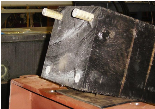
Figure (3.11): a) Displacement at the supports, b) Displacement at the mid span, c) Slippage of GFRP Rebars
