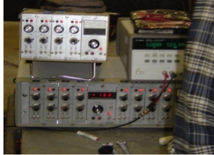
Figure (2.11): Load, deflection and strain data continuously and automatically recorded using a computerized data acquisition system
