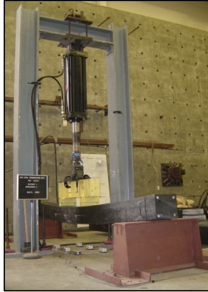
Figure (2.13): Typical 4-point beam test setup
