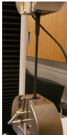
Figure (2.4): Specimen Tensile testing in Instron 3367
