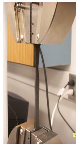
Figure (2.4): Specimen Tensile testing in Instron 3367
