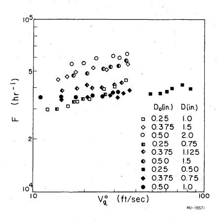
Fig. 8. Effect of hole diameter and spacing on frequency. (Air-water system,  $V_c = 262 \text{ in}^3$ ., n = 3,  $h_L = 2.0 \text{ in}$ .)
