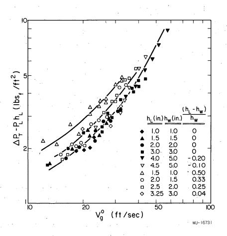
Fig. 55. Pressure-drop data for two-ft-column.
