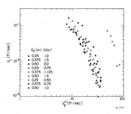
Fig. 45. Effect of hole diameter and spacing on multihole dumping rates. (Air-water system,  $V_c = 262 \text{ in}^3$ ., n = 3,  $h_L = 2.0 \text{ in}$ .)
