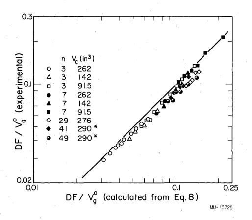
Fig. 12. Correlation of effect of chamber volume on frequency. (Air-water system,  $h_L$  = 2.0 in.,  $D_o$  = 0.25 in., D = 1.0 in., D = 0.75 in.)
