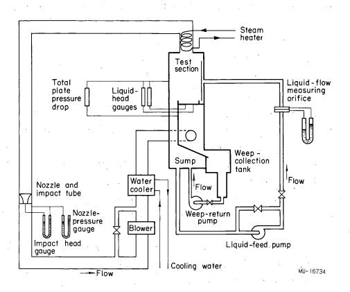
Fig. 48. Schematic diagram of 2-ft. column.
