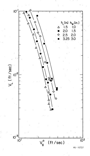
Fig. 51. Dumping data for 2-ft. column. (Air-water system,  $h_L > h_w$ ).
