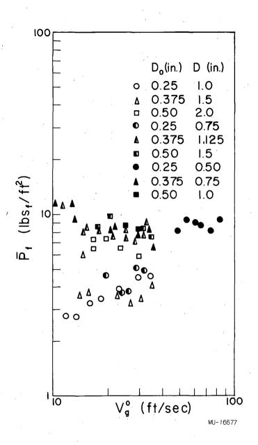
Fig. 21. Effect of hole diameter and spacing on average amplitude of pressure fluctuations. (Air-water system,  $V_c = 262 \text{ in}^3$ ., n = 3,  $h_L = 2.0 \text{ in}$ .)
