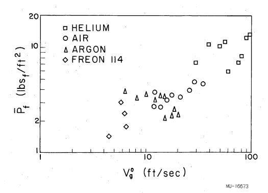
Fig. 15. Effect of gas properties on average amplitude of pressure fluctuations. (Water as liquid,  $V_c = 262 \text{ in}^3$ .,  $D_o = 0.25 \text{ in.}$ , D = 1.0 in., n = 3,  $h_L = 2.0 \text{ in.}$ )
