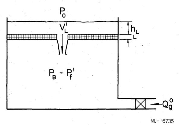
Fig. 40. Schematic diagram of single-hole dumping.
