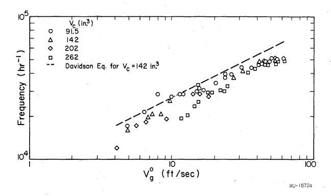
Fig. 10. Single-hole frequency. (Air-water system,  $D_0 = 0.25 \text{ in.}$ )
