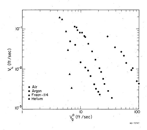
Fig. 43. Effect of gas properties on multihole dumping rates. (Water as liquid,  $V_c = 262 \text{ in}^3$ .,  $D_o = 0.25 \text{ in.}$ , D = 1.0 in., n = 3,  $h_L = 2.0 \text{ in.}$ )
