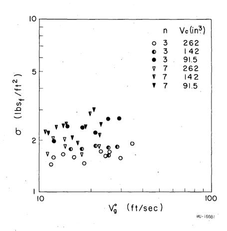
Fig. 29. Effect of chamber volume and number of holes on standard deviation of pressure fluctuations. (Air-water system,  $D_0 = 0.25$  in., D = 1.0 in.,  $h_L = 2.0$  in.)
