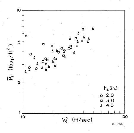
Fig. 16. Effect of liquid head on average amplitude of pressure fluctuations. (Air-water system,  $V_c = 262 \text{ in}^3$ ., n = 3,  $D_o = 0.25 \text{ in.}$ , D = 1.0 in.,  $h_L = 2.0 \text{ in.}$ )
