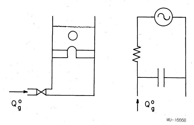
Fig. 5. Electrical analog to bubbling.
