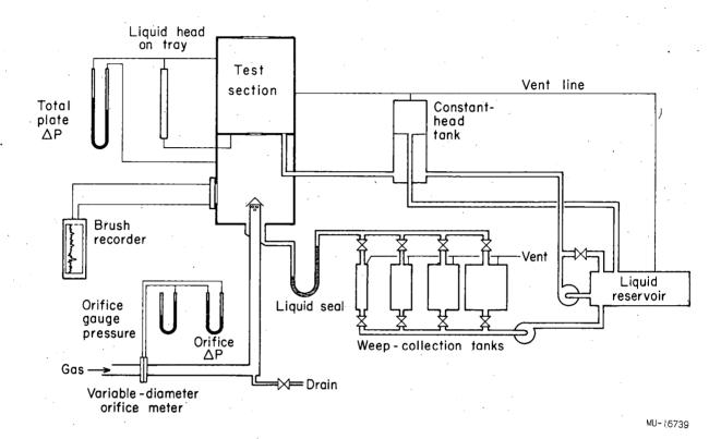
Fig. 1. Schematic diagram of 6-in. column.
