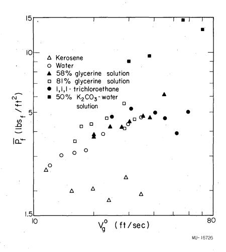
Fig. 17. Effect of liquid properties on average amplitude of pressure fluctuations. (Air as gas,  $V_c = 262 \text{ in}^3$ ., n = 3,  $D_o = 0.25 \text{ in.}$ , D = 1.0 in.,  $h_L = 2.0 \text{ in.}$ )
