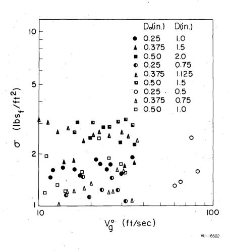
Fig. 30. Effect of hole diameter and spacing of standard deviation of pressure fluctuations. (Air-water system,  $V_c = 262 \text{ in}^3$ ., n = 3,  $h_L = 2.0 \text{ in}$ .)
