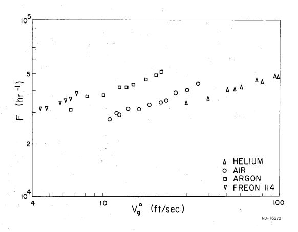
Fig. 7. Effect of gas properties on frequency. (Water as liquid,  $V = 262 \text{ in}^3$ .,  $h_L = 2.0 \text{ in.}$ ,  $D_0 = 0.25 \text{ in.}$ , n = 3, D = 1.0 in.)
