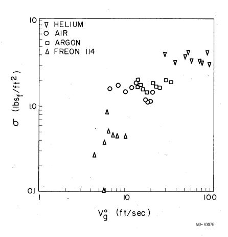
Fig. 27. Effect of gas properties on standard deviation of pressure fluctuations. (Water as liquid,  $D_0$  = 0.25 in., D = 1.0 in.,  $V_c$  = 262 in<sup>3</sup>., n = 3,  $h_L$  = 2.0 in.)
