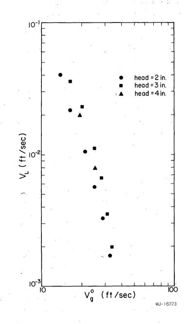
Fig. 46. Effect of head on multihole dumping rates. (Air-water system,  $V_c = 262 \text{ in}^3$ .,  $D_o = 0.25 \text{ in.}$ , D = 1.0 in., n = 3.)
