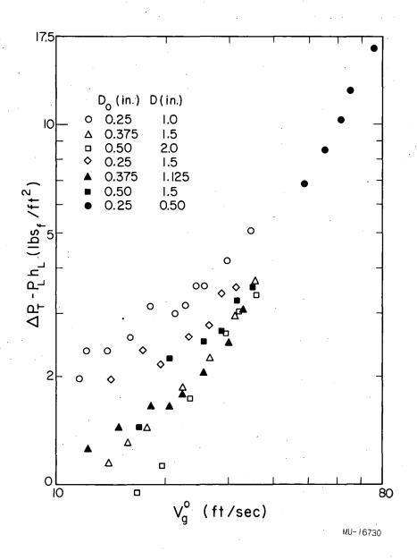
Fig. 32. Effect of hole diameter and spacing on pressure drop. (Air-water system,  $V_c = 262 \text{ in}^3$ ., n = 3,  $h_L = 2.0 \text{ in.}$ )
