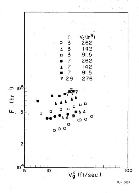
Fig. 6. Effect of chamber volume on frequency. (Air-water system,  $D_0 = 0.25$  in., D = 1.0 in.,  $h_L = 2.0$  in.)
