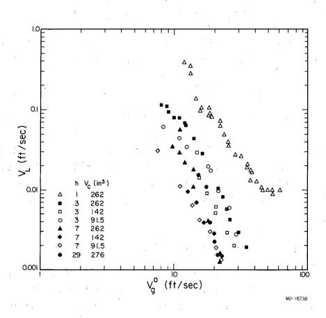
Fig. 47. Effect of chamber volume and number of holes on multihole dumping rates. (Air-water system,  $D_0 = 0.25$  in., D = 1.0 in.,  $h_L = 2.0$  in.)
