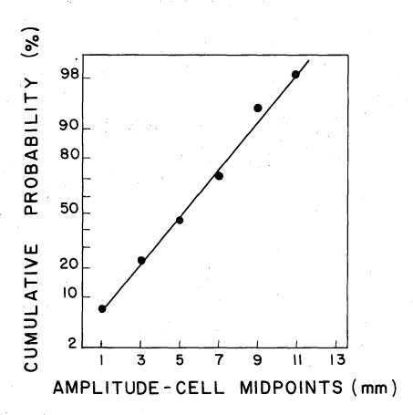
Fig. 26. Test of normality - multihole plate. (Air-water system,  $V_0^o$  = 29.8 ft/sec.,  $V_c$  = 262 in<sup>3</sup>.,  $D_o$  = 0.25 in., D = 1.0 in., n = 3,  $h_L$  = 2.0 in.)
