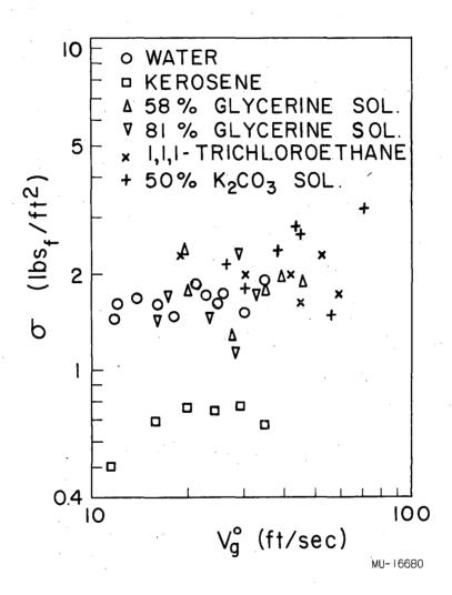
Fig. 28. Effect of liquid properties on standard deviation of pressure fluctuations. ( $V_c = 262 \text{ in}^3$ .,  $D_o = 0.25 \text{ in}$ ., D = 1.0 in., n = 3,  $h_L = 2.0 \text{ in.}$ , air as gas)
