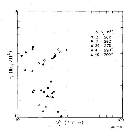
Fig. 20. Multihole data - Effect of number of holes on average amplitude of pressure fluctuations. (Air-water system, D<sub>o</sub> = 0.25 in., D = 1.0 in., h<sub>L</sub> = 2.0 in., \*D = 0.75 in.)
