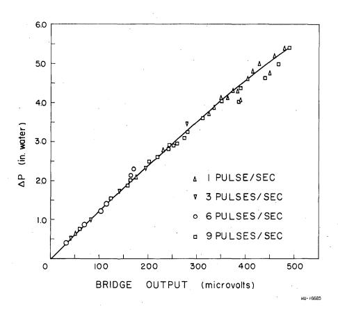
Fig. 57. Strain-gauge diaphragm calibration.
