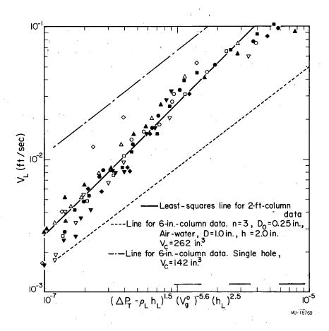
Fig. 54. Proposed correlation for 2-ft-column dumping data. ( $\Delta P_t - p_L h_L$  in lb/ft<sup>2</sup>,  $V_g^o$  in ft/sec,  $h_L$  in inches of water.)
