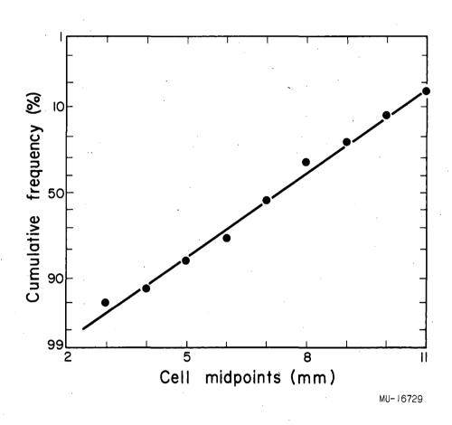
Fig. 24. Test of normality - single-hole plate. (Air-water system, V = 91.5 in<sup>3</sup>., D<sub>o</sub> = 0.25 in., h<sub>L</sub> = 2.0 in., V<sub>g</sub> = 31 ft/sec).
