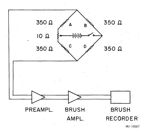
Fig. 2. Pressure-fluctuation measuring circuit. (Bridge powered by 7 Mallory 4 RM-4R batteries.)
