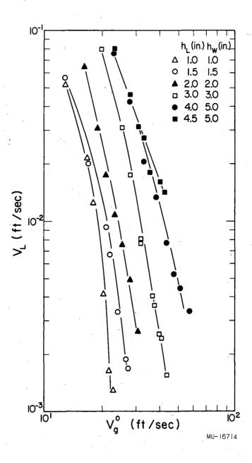
Fig. 52. Dumping data for 2-ft. column. (Air-water system,  $h_{1} \le h_{w}$ ).
