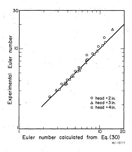
Fig. 38. Effect of liquid head on Euler Number. (Air-water system,  $V_c = 262 \text{ in}^3$ .,  $D_o = 0.25 \text{ in.}$ , D = 1.0 in., n = 3.)
