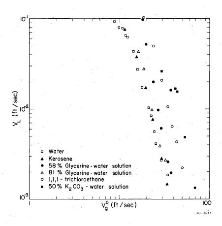
Fig. 44. Effect of liquid properties on multihole dumping rates. (Air as gas,  $V_c = 262 \text{ in}^3$ .,  $D_o = 0.25 \text{ in.}$ , D = 1.0 in., n = 3,  $h_L = 2.0 \text{ in.}$ )
