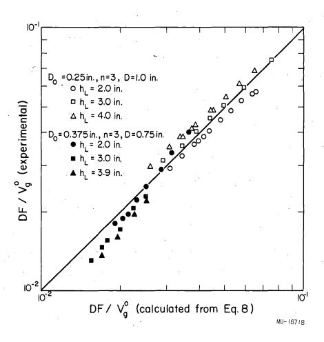
Fig. 13. Correlation of liquid-head effect on frequency. (Air-water system,  $V_c = 262 \text{ in}^3$ .)
