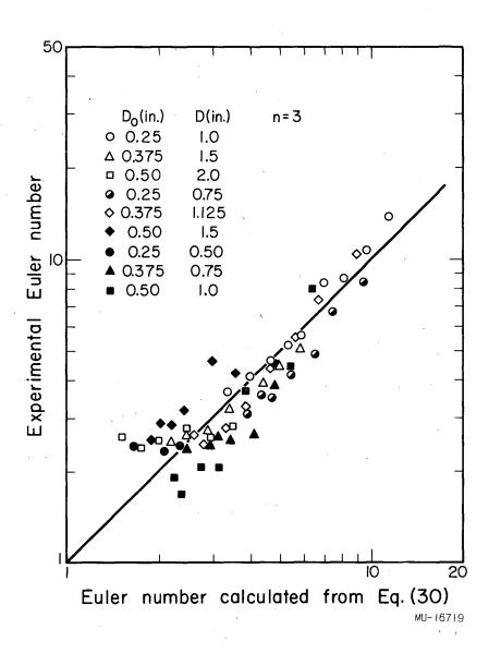
Fig. 37. Correlation of effect of hole diameter and spacing on pressure drop. (Air-water system,  $V_c = 262 \text{ in}^3$ ., n = 3,  $h_L = 2.0 \text{ in.}$ )
