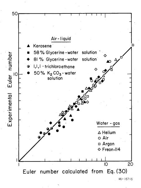
Fig. 36. Correlation of effects of gas and liquid properties on pressure drop.  $(V_c = 262 \text{ in}^3., D_o = 0.25 \text{ in.}, D = 1.0 \text{ in.}, n = 3, h_L = 2.0 \text{ in.})^c$
