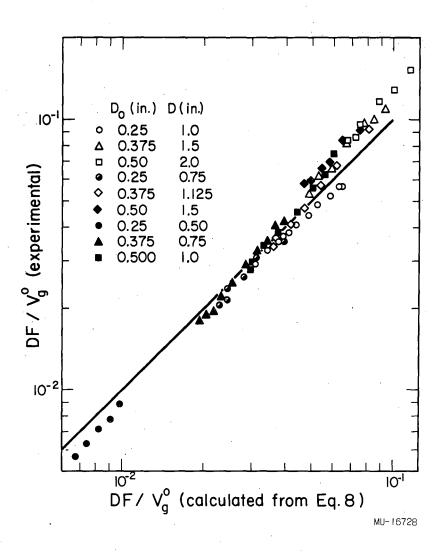
Fig. 14. Correlation of effect of hole diameter and spacing on frequency. (Air-water system,  $V_c = 262 \text{ in}^3$ ., n = 3,  $h_L = 2.0 \text{ in.}$ )
