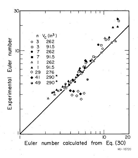
Fig. 39. Correlation of effect of chamber volume on pressure drop. (Air-water system,  $D_0$  = 0.25 in., D = 1.0 in.,  $h_L$  = 2.0 in., D = 0.75 in.
