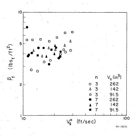
Fig. 18. Effect of chamber volume and number of holes on average amplitude of pressure fluctuations. (Air-water system,  $D_0$  = 0.25 in., D = 1.0 in.,  $h_L$  = 2.0 in.)
