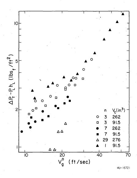
Fig. 33. Effect of chamber volume on pressure drop. (Air-water system,  $D_0$  = 0.25 in., D = 1.0 in.,  $h_L$  = 2.0 in.)
