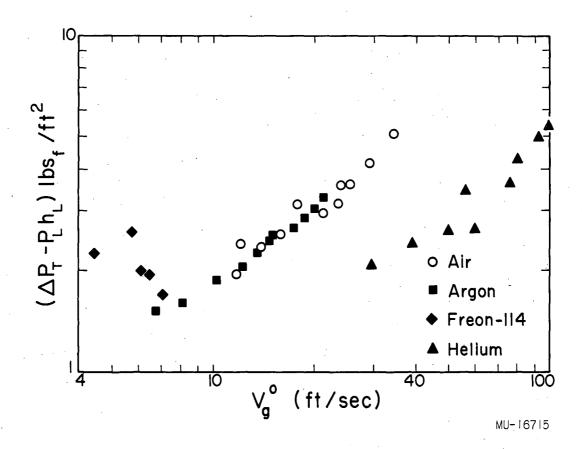
Fig. 35. Effect of gas properties on pressure drop. (Water as liquid,  $V_c$  = 262 in<sup>3</sup>.,  $D_o$  = 0.25 in., D = 1.0 in., n = 3,  $h_L$  = 2.0 in.)
