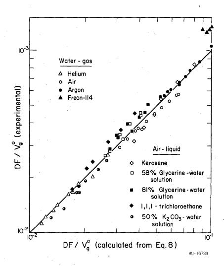
Fig. 11. Correlation of effects of gas and liquid properties on frequency. ( $V_c = 262 \text{ in}^3$ .,  $D_o = 0.25 \text{ in}$ ., D = 1.0 in.,  $h_L = 2.0 \text{ in}$ .)
