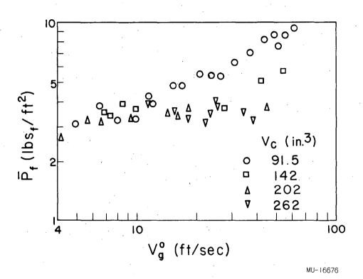
Fig. 19. Single hole data - Effect of chamber volume on average amplitude of pressure fluctuations. (Air-water system,  $D_0 = 0.25$  in.,  $h_L = 2.0$  in.)
