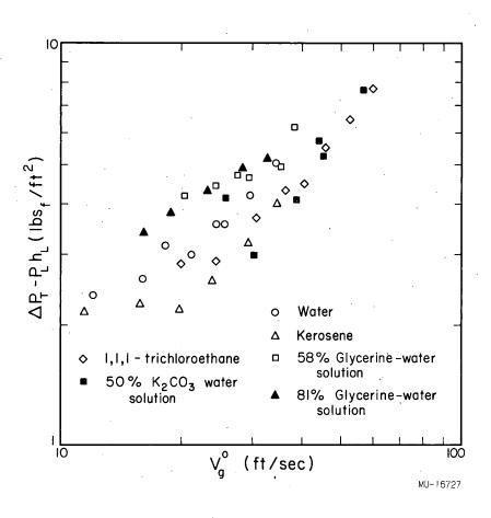
Fig. 34. Effect of liquid properties on pressure drop. (Air as gas,  $V_c = 262 \text{ in}^3$ .,  $D_o = 0.25 \text{ in.}$ , D = 1.0 in., n = 3,  $h_L = 2.0 \text{ in.}$ )
