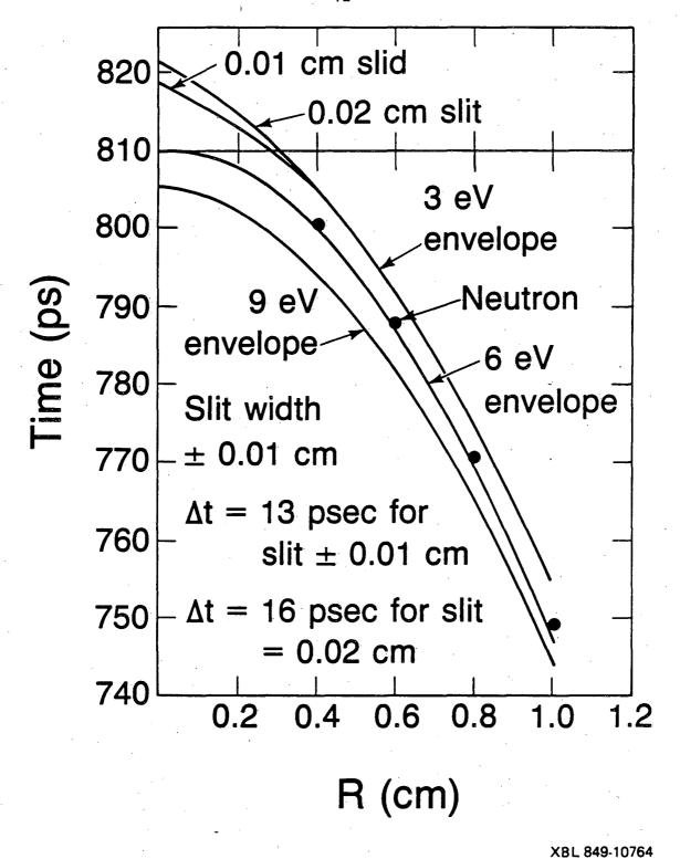
Fig. 2. Transit times versus radial emission point.
