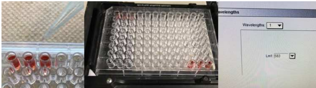
Figure A.7: Measuring the absorbance intensity of Cbi solution.
