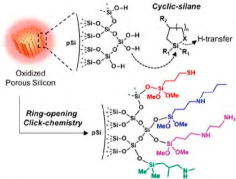
Figure 1.6: Schematic of ring-opening “click” reactions of heterocyclic silanes to graft various functional groups onto the surface of porous silicon oxides. 13
