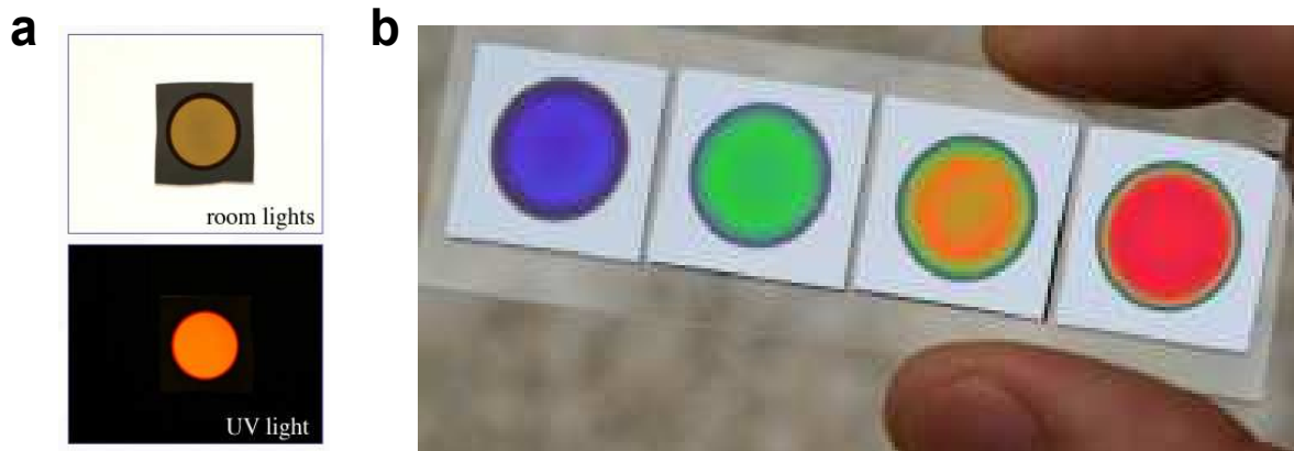
Figure 1.2: Unique optical properties of porous silicon. (a) pSi displays photoluminescent properties which can enable the material to display a red-orange color when illuminated with a UV-light. 1 (b) pSi can also be tuned to make photonic crystal structures that can display various colors within the visible spectrum. 1
