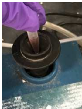
Figure A.5: Vortexing pSiMPs to remove Cbi from the particles.
