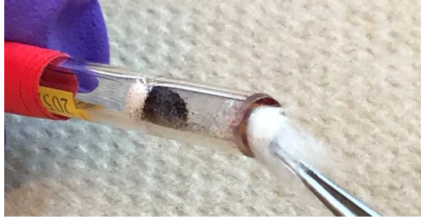
Figure A.2: Removing Cbi-loaded pSiMPs from thermal desorption tube.
