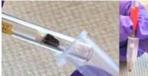
Figure A.3: Transferring Cbi-loaded pSiMPs into Eppendorf™ □ tube.
