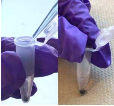
Figure A.4: Adding ethanol to Cbi-loaded pSiMPs.
