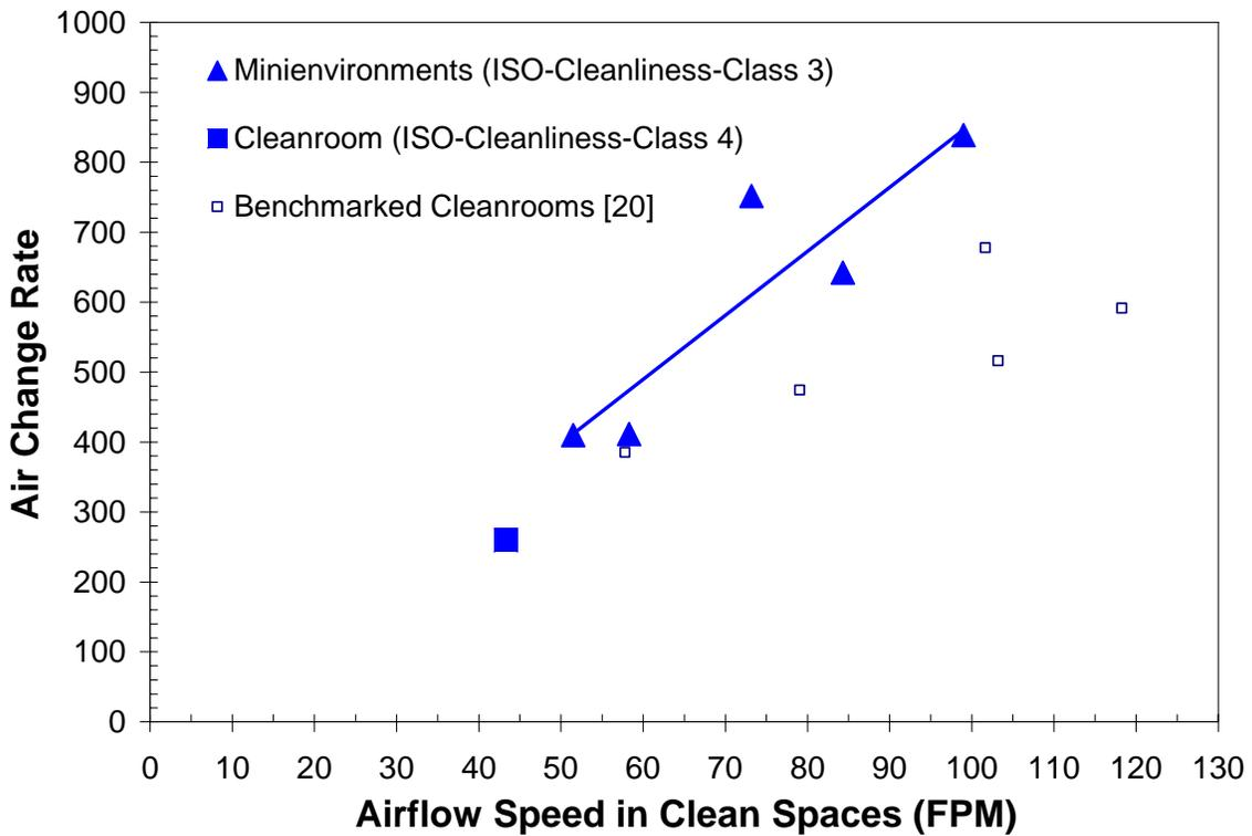
**Figure 1 Air Change Rates and Airflow Speed**
