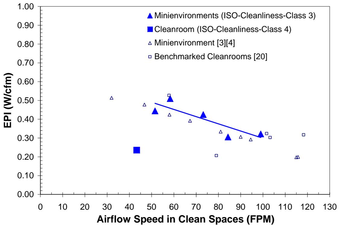
**Figure 2 Energy Performance Index and Airflow Speed**
